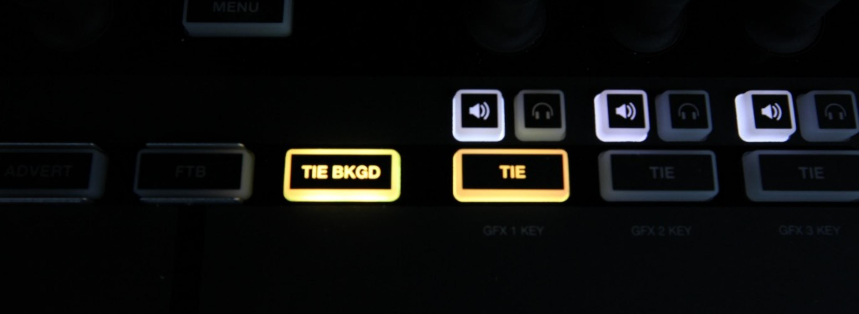
To both switch the video source and bring in a graphics overlay at the same time, select '**TIE BKGD**' and the corresponding **TIE** button for your graphic.
