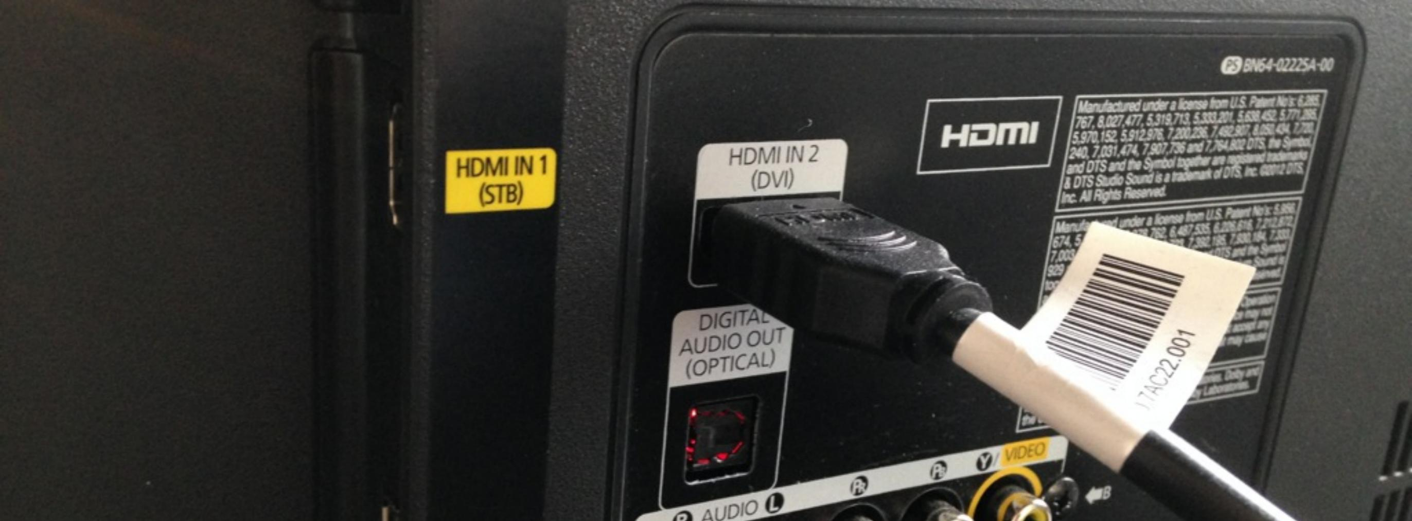
Run the cable to your output source and connect it to the proper input port.
