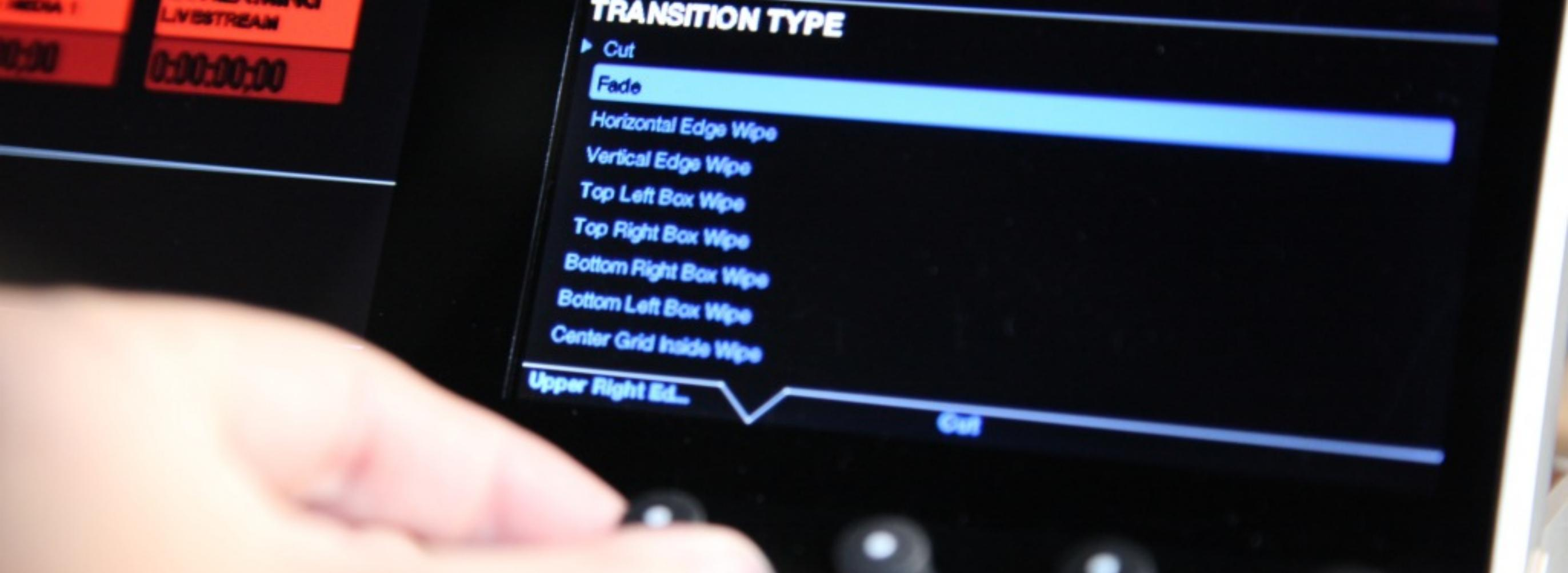
On the right monitor, you will have the option to select different transitions for your three graphics overlay channels. Press and turn the corresponding knobs to do this.
