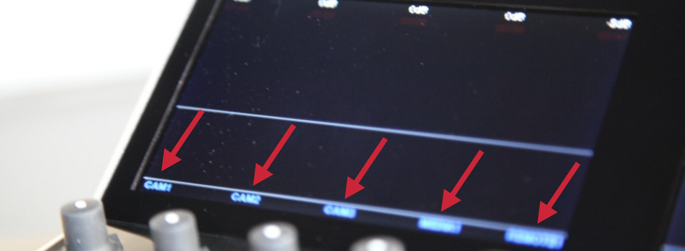
On the left monitor, you should notice that the names of your 5 input sources appear on the bottom of the screen.
