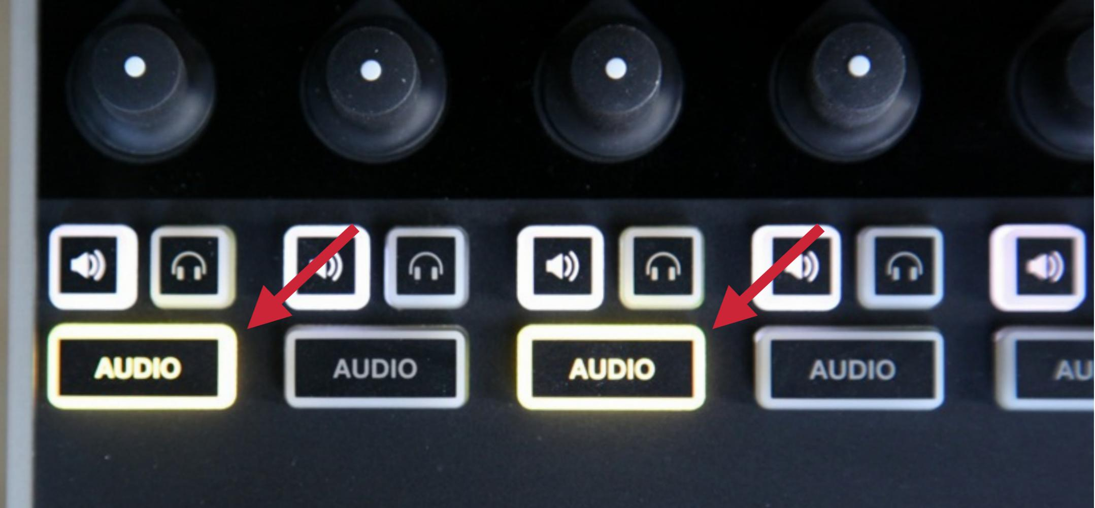
When either source is in Program, both audio control buttons will light up, indicating that both sources have the same audio.
