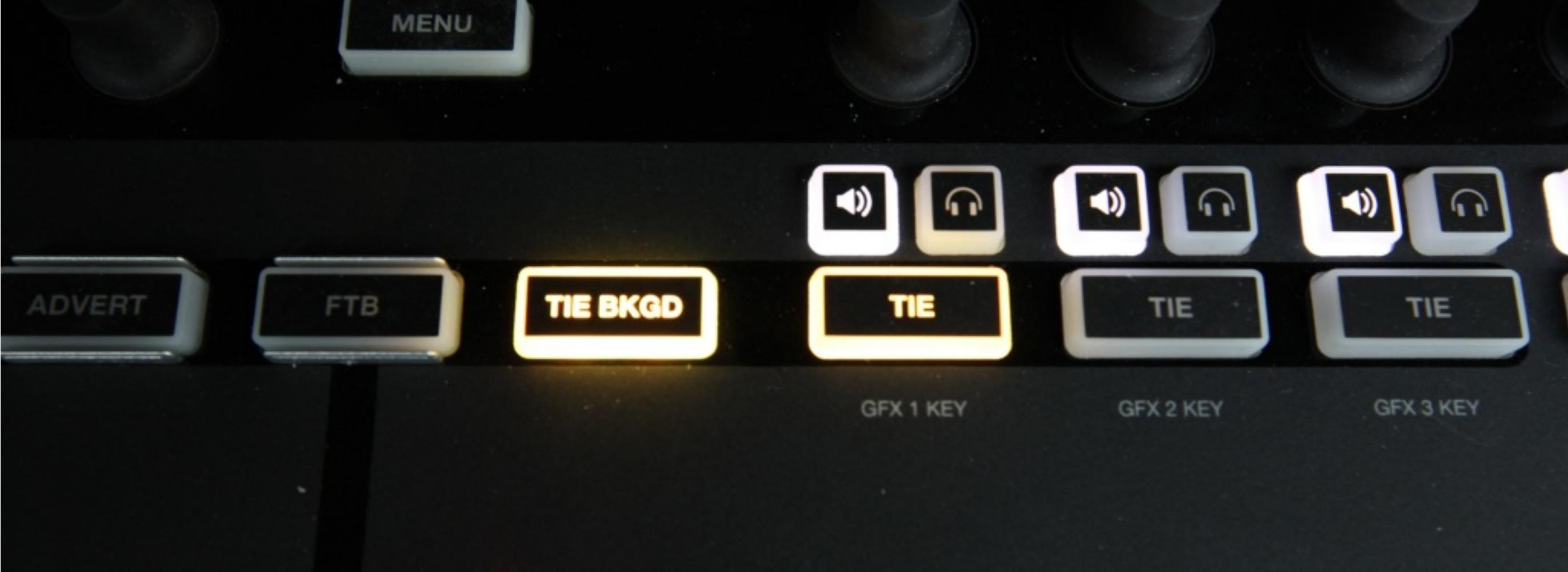
To pull a graphics overlay out of Program simultaneously with a video source, tie the background and the graphics overlay together.
