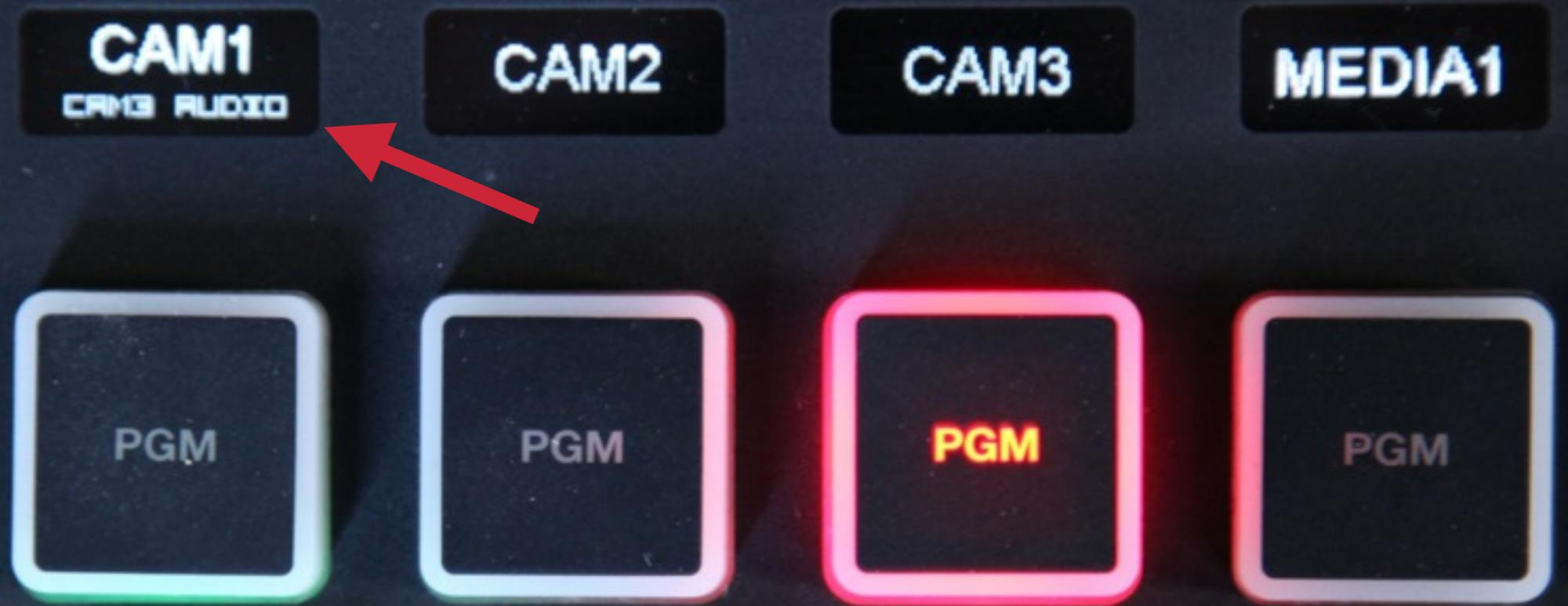
You will know which audio source is being used by checking the track assignment labels, which tell you where audio is coming from for a linked source.
