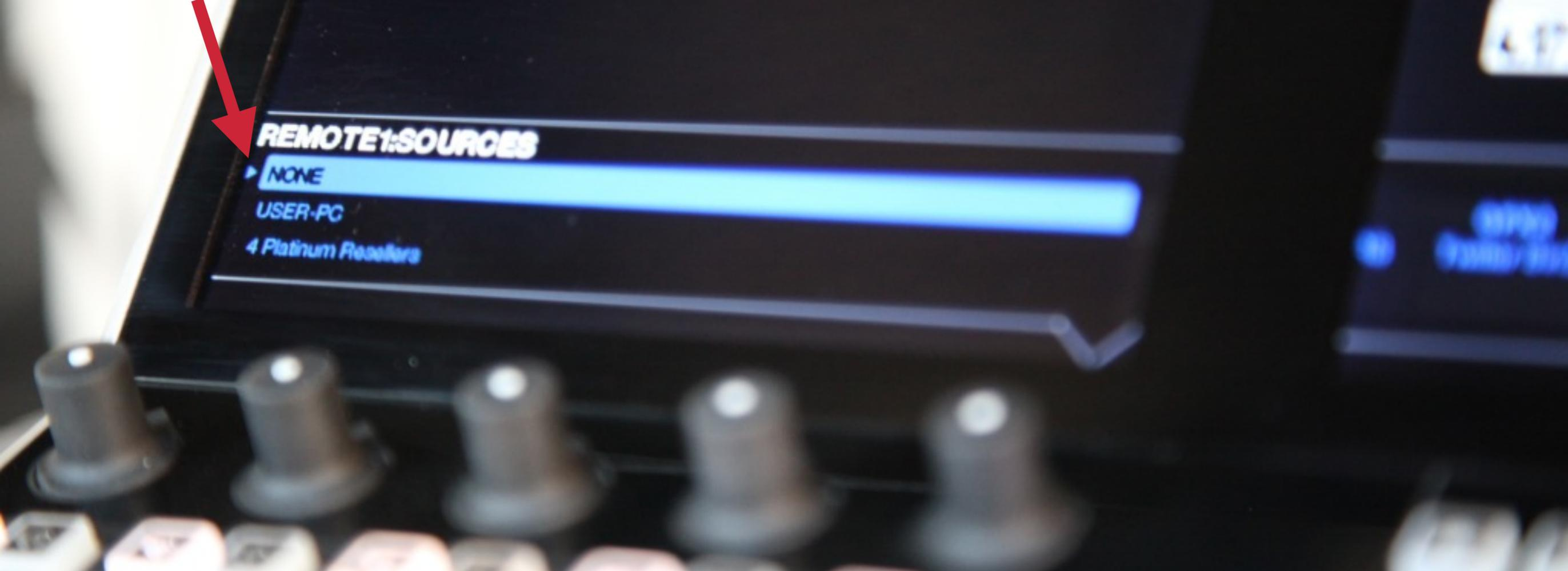
The left arrow indicates which source is currently being seen in the remote camera module.
