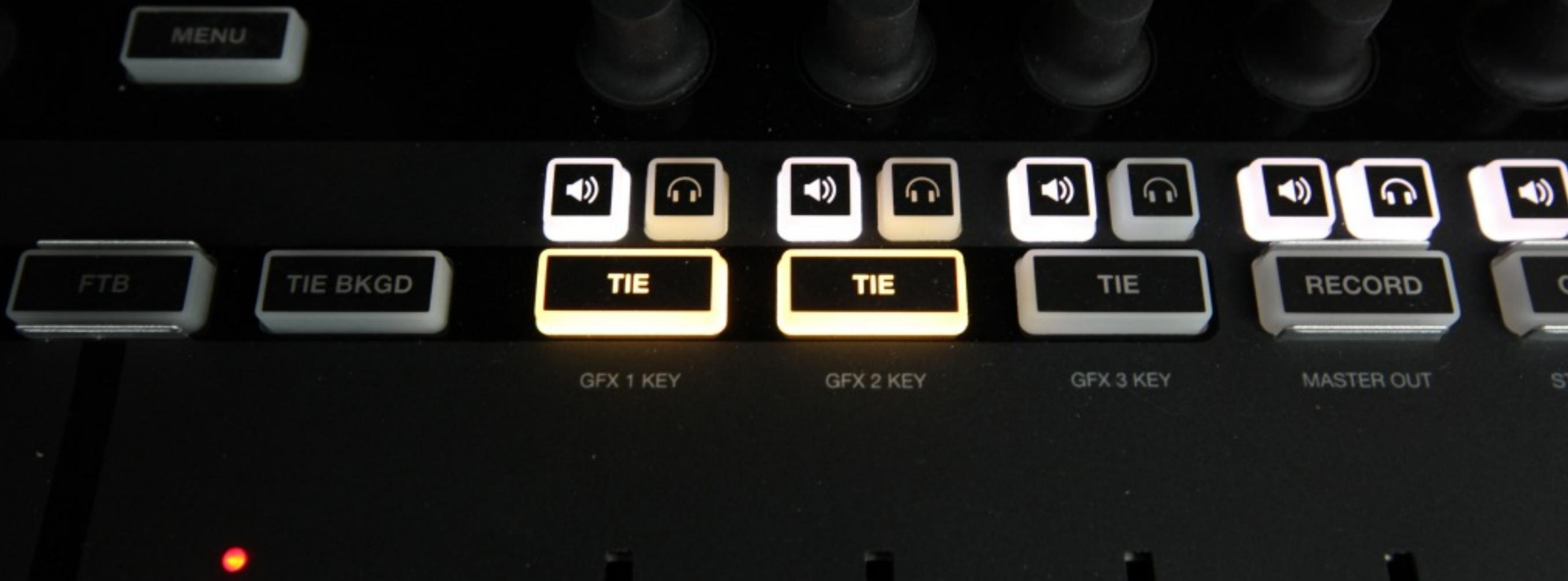
If only the GFX 1 and GFX 2 **'TIE'** buttons are lit and both sources are in Preview, then both overlays will switch into Program when transitioning. The video will not change.
