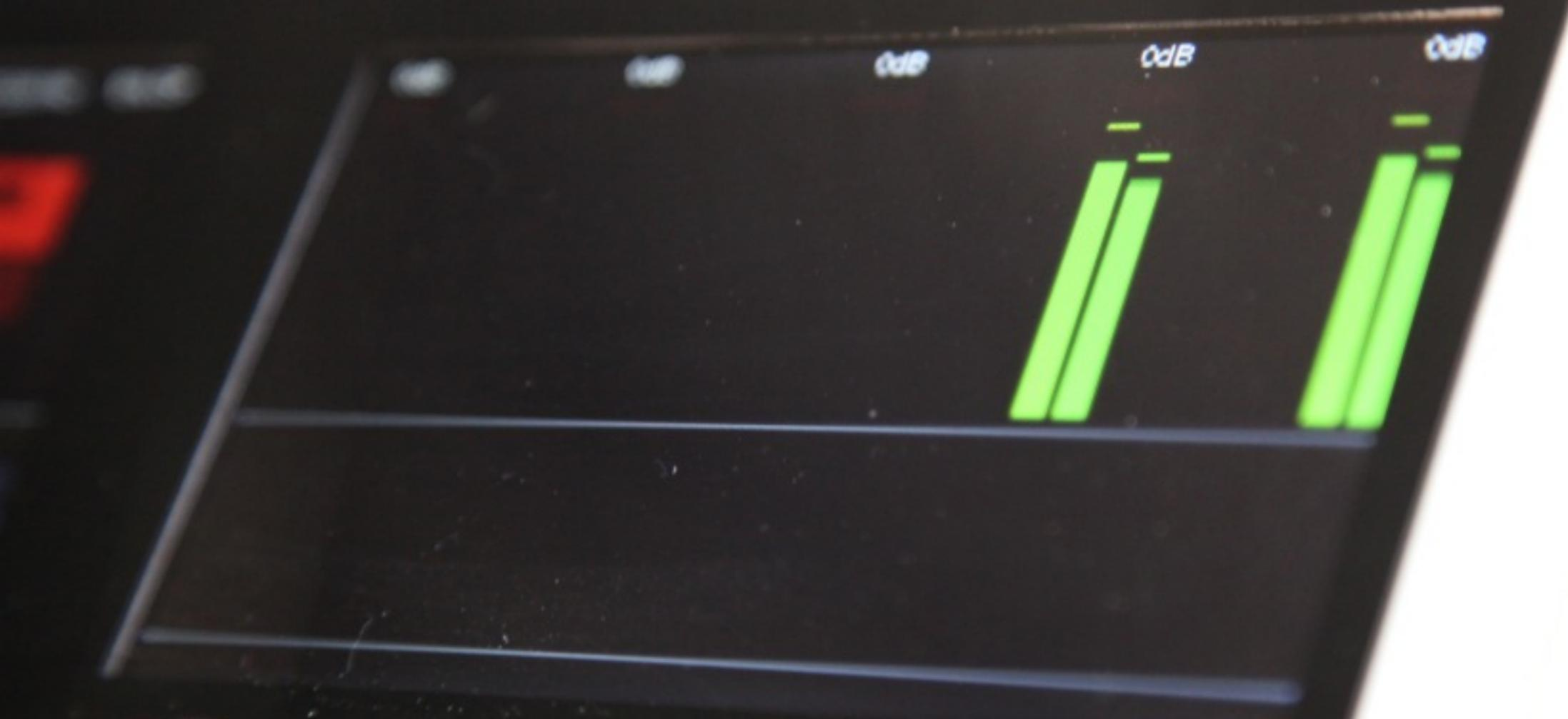
The upper right monitor shows audio levels for the graphics overlays, Program record, and Program stream.
