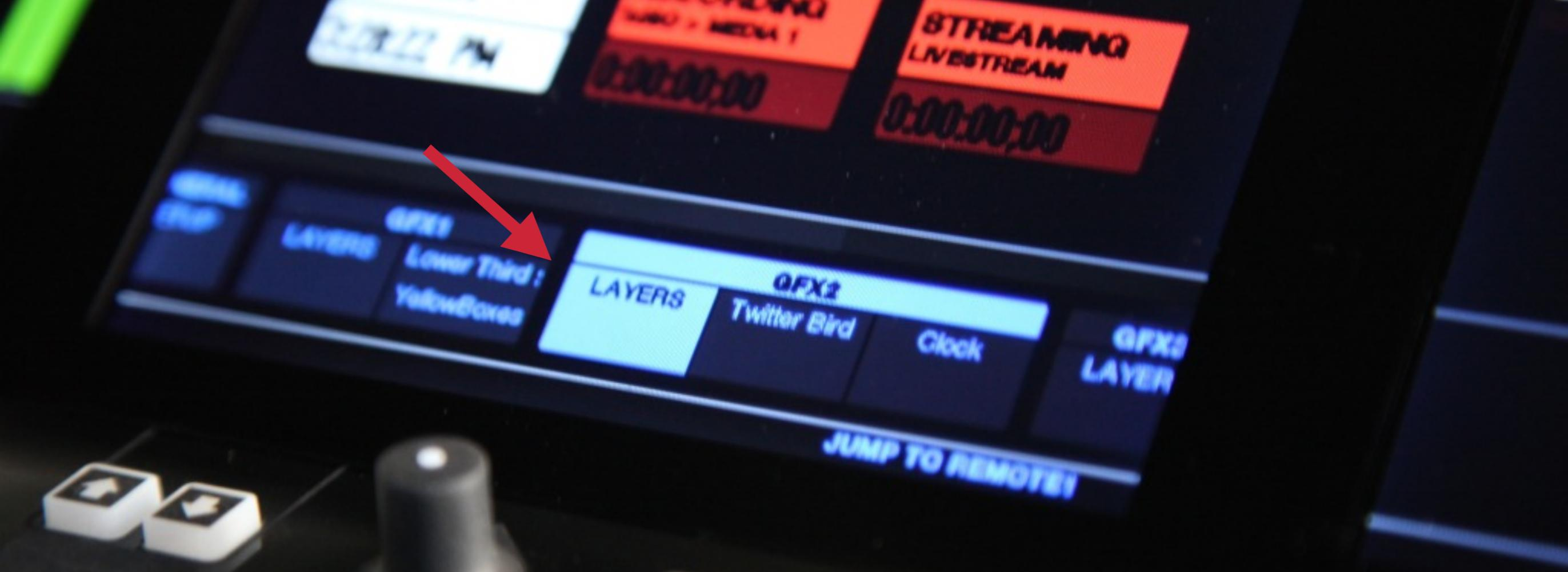
One type of assignment you can set is for viewing all the layers within that graphics channel. First, select the layers menu within that channel.
