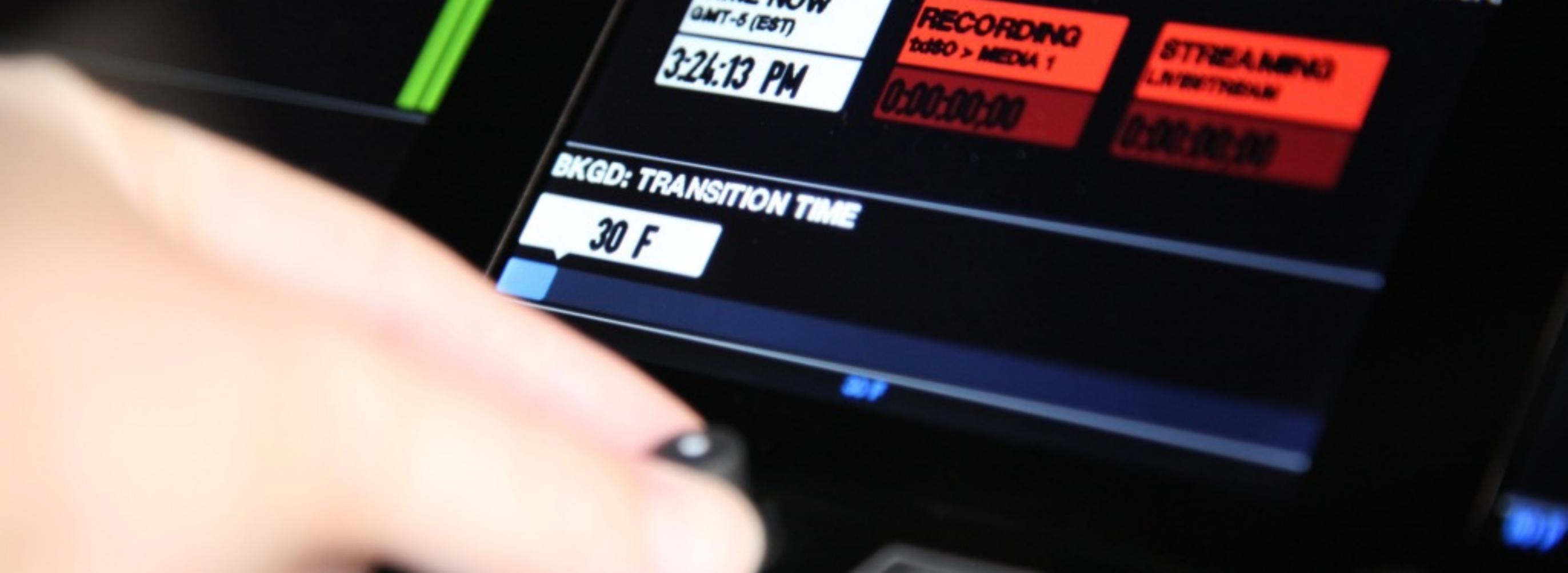
Turn and press the knob to determine how many frames you want an automatic transition to utilize (i.e., pressing '**Auto**' to switch Preview and Program).
