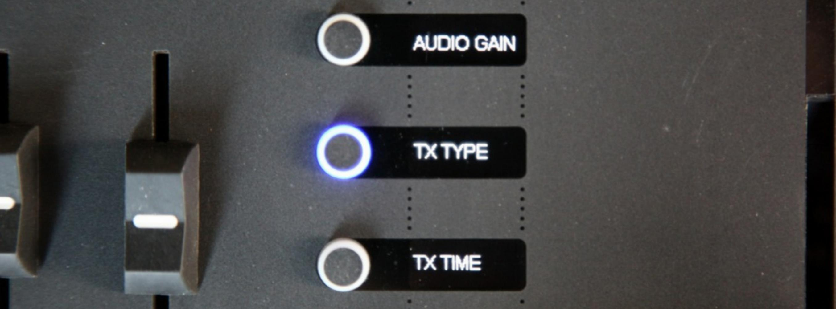
The fourth General Setup menu option is '**TX TYPE**,' which is an abbreviation for Transition Type.
