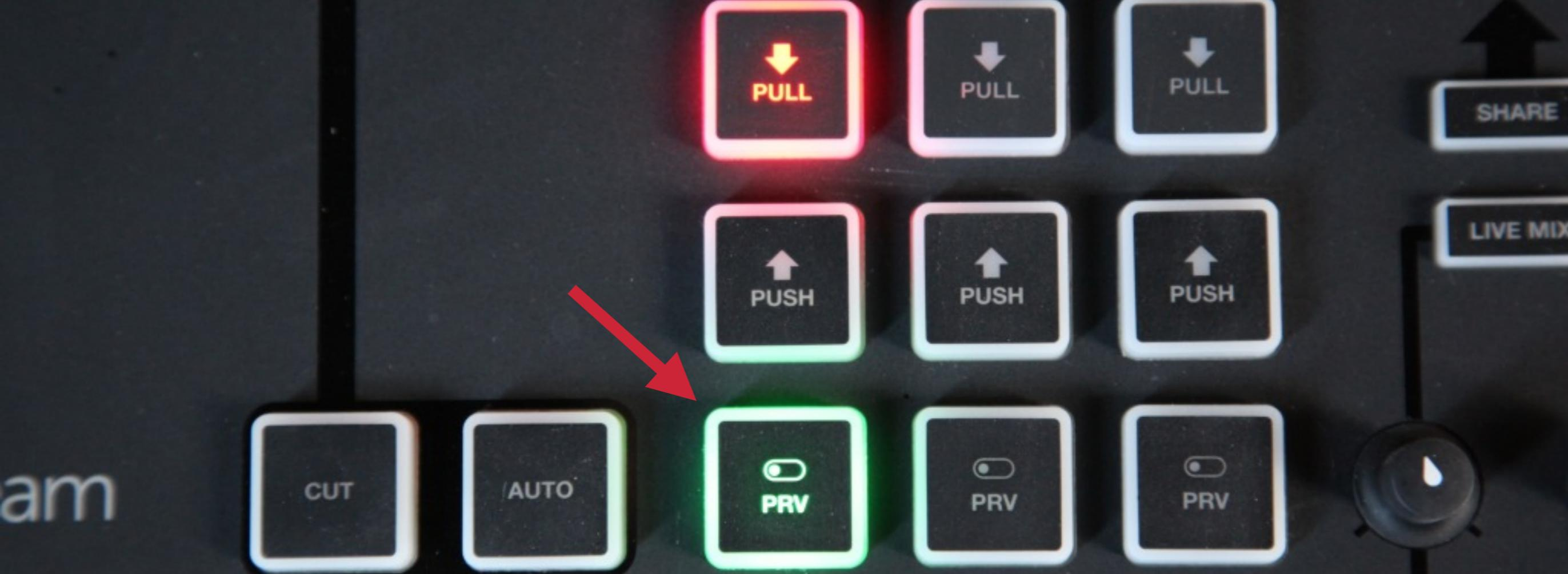
Next, you will need to remove the graphics overlay from Preview. This will tell the transition controls that the graphic is not being shown on the next switch.
