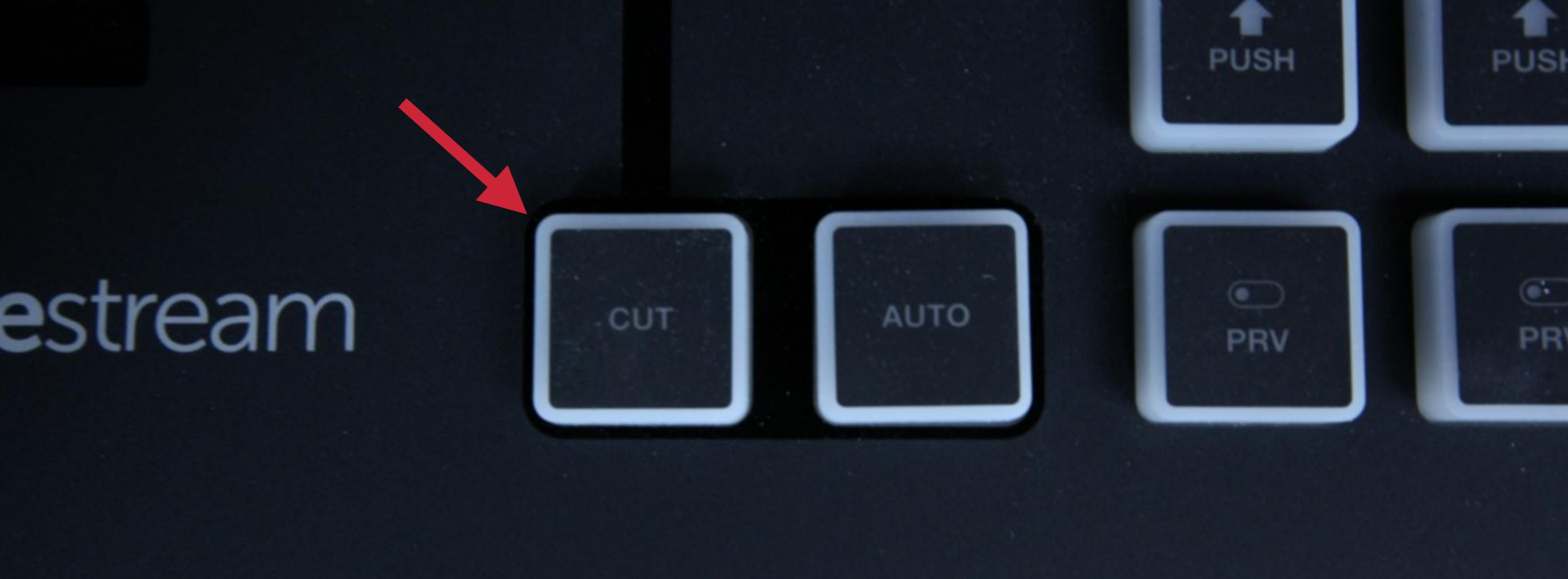
One transition type is **cut**, which switches Preview & Program with no overlap between the sources. To do this transition, press the '**Cut**' button.
