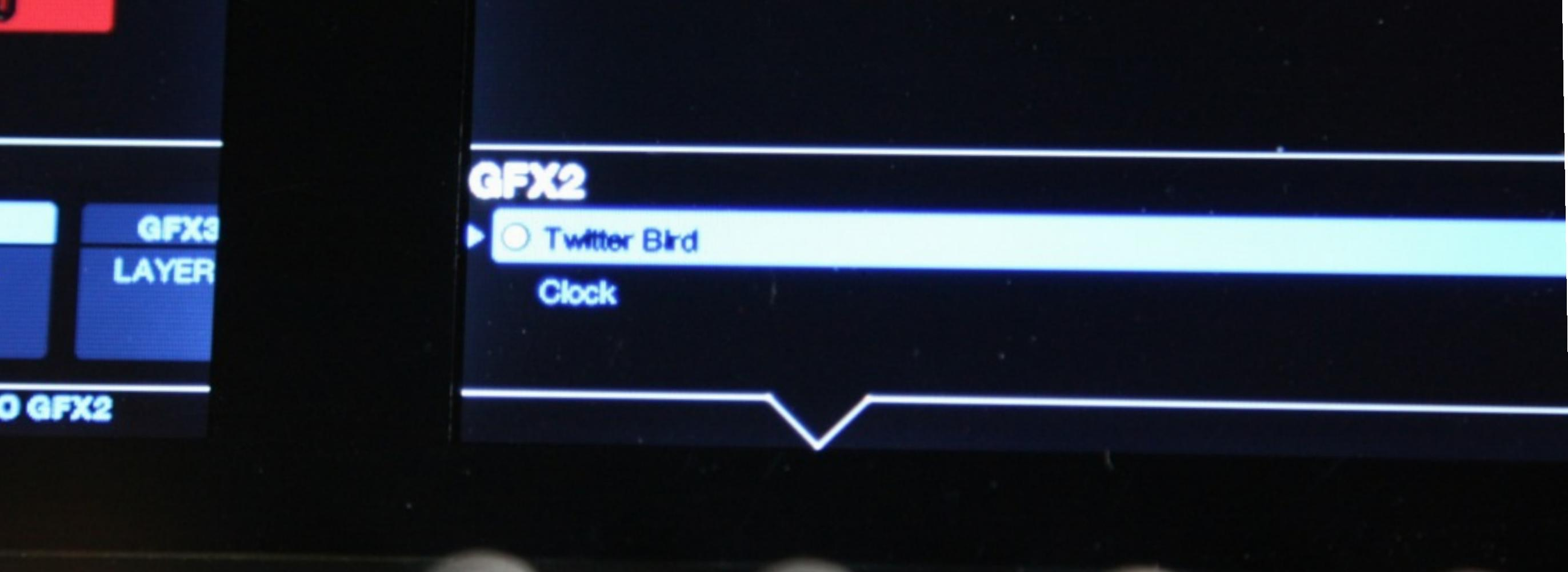
Turning the knob will show the names of all the layers within that graphics overlay channel.
