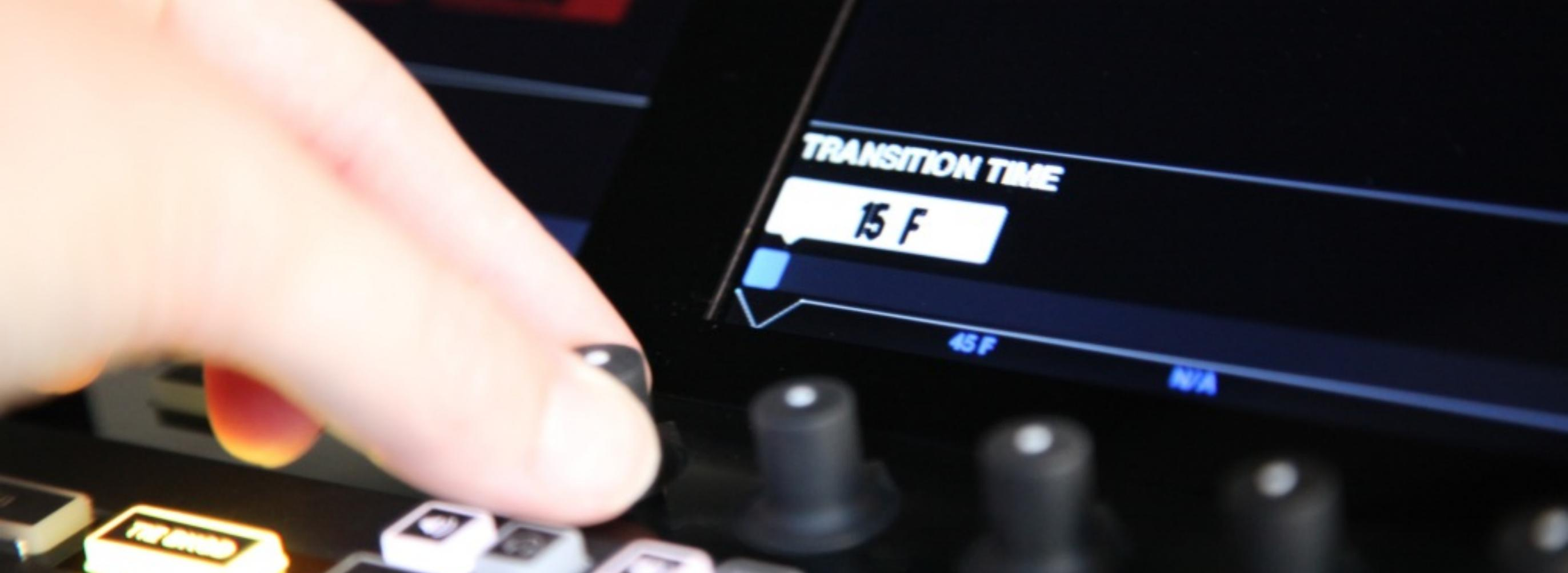
Just as with transition type, the main mix and the three graphics overlay channels can have independently set transition times. (**Cut** cannot have a set time.)
