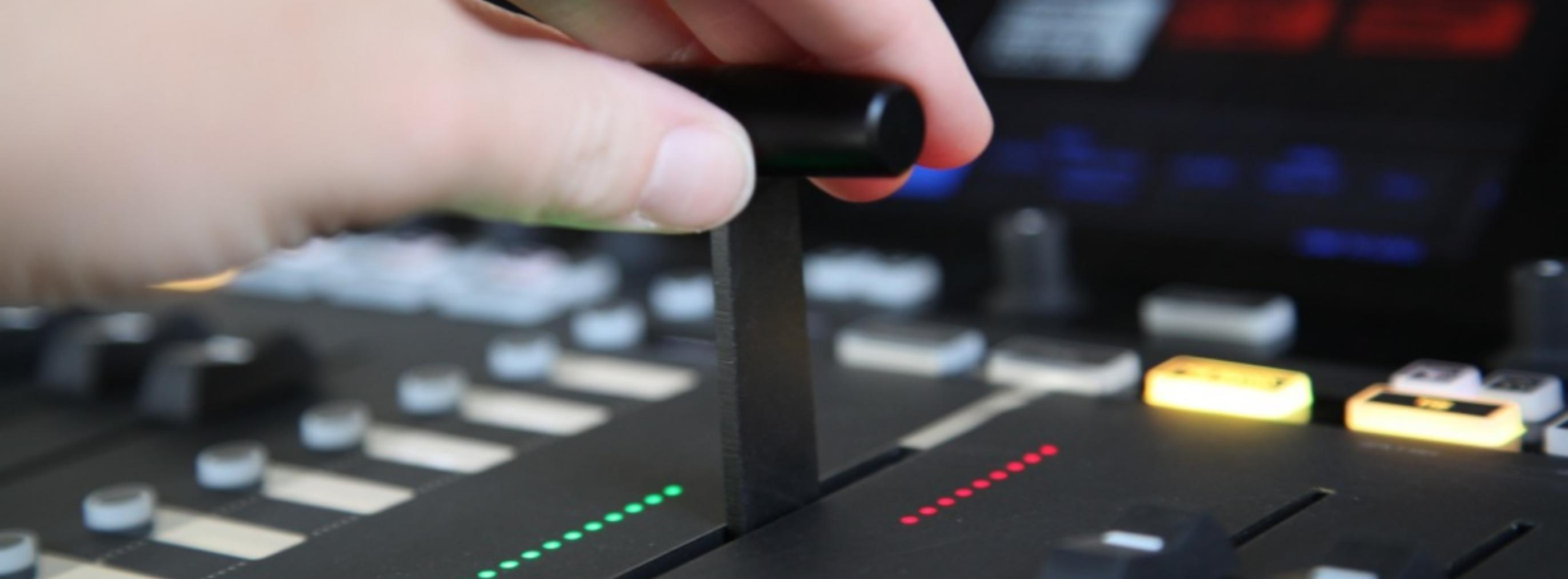
Another way to use that transition is to manually switch your sources using the **T Bar** on the Studio Surface. This allows you to control the transition's speed.
