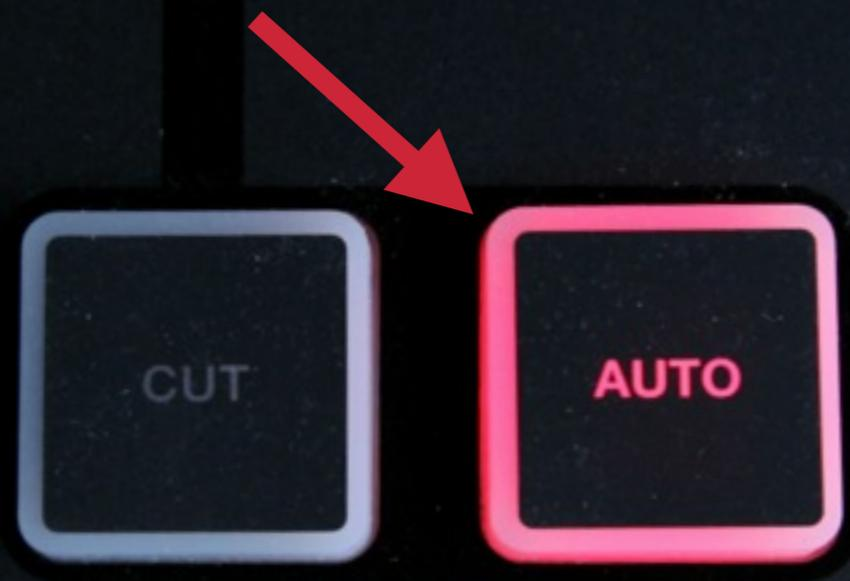
One way to activate the fade or wipe transition is by pressing the '**Auto**' button, which will perform the switch at the speed you set under the Transitions menu.
