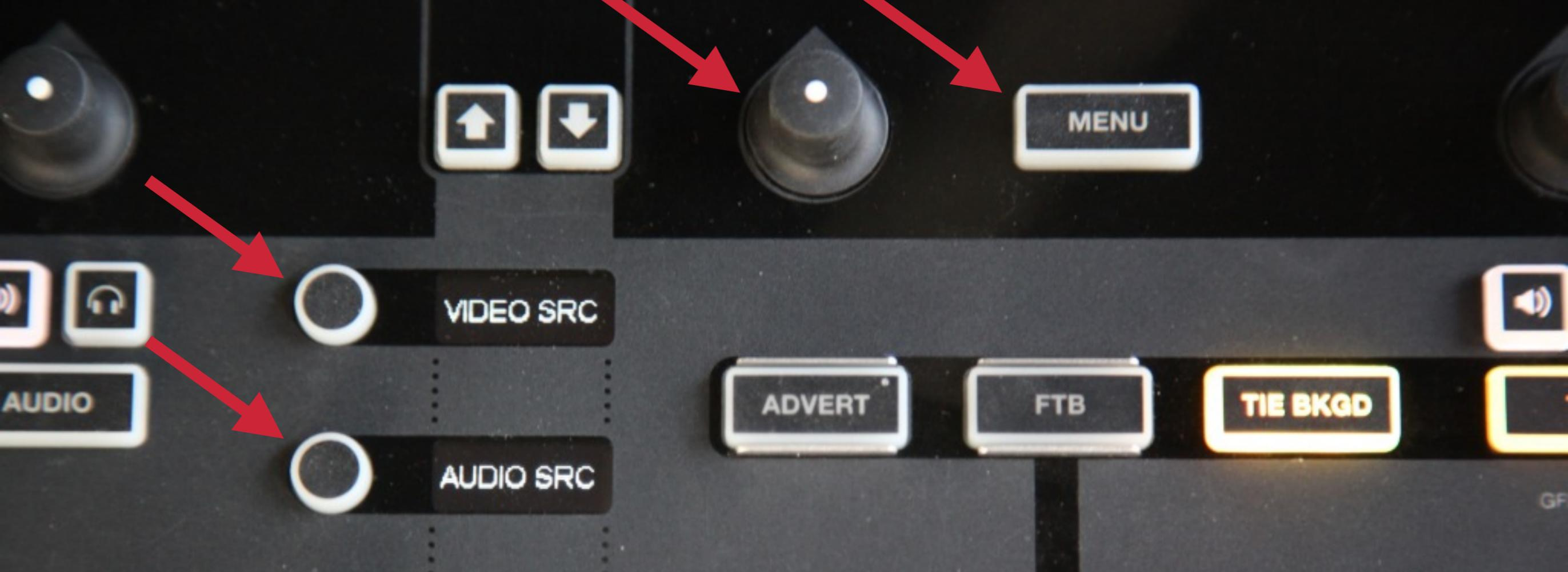
The controls for these menus include the knob below the monitor and the **menu buttons** running down the center of the Studio Surface.
