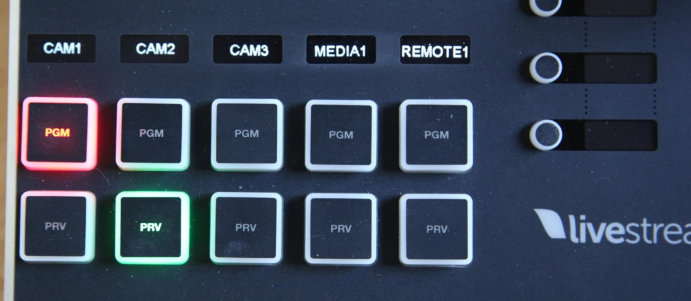
The bottom left corner has the Preview (**PRV**) and Program (**PGM**) controls for 5 assigned input sources.
