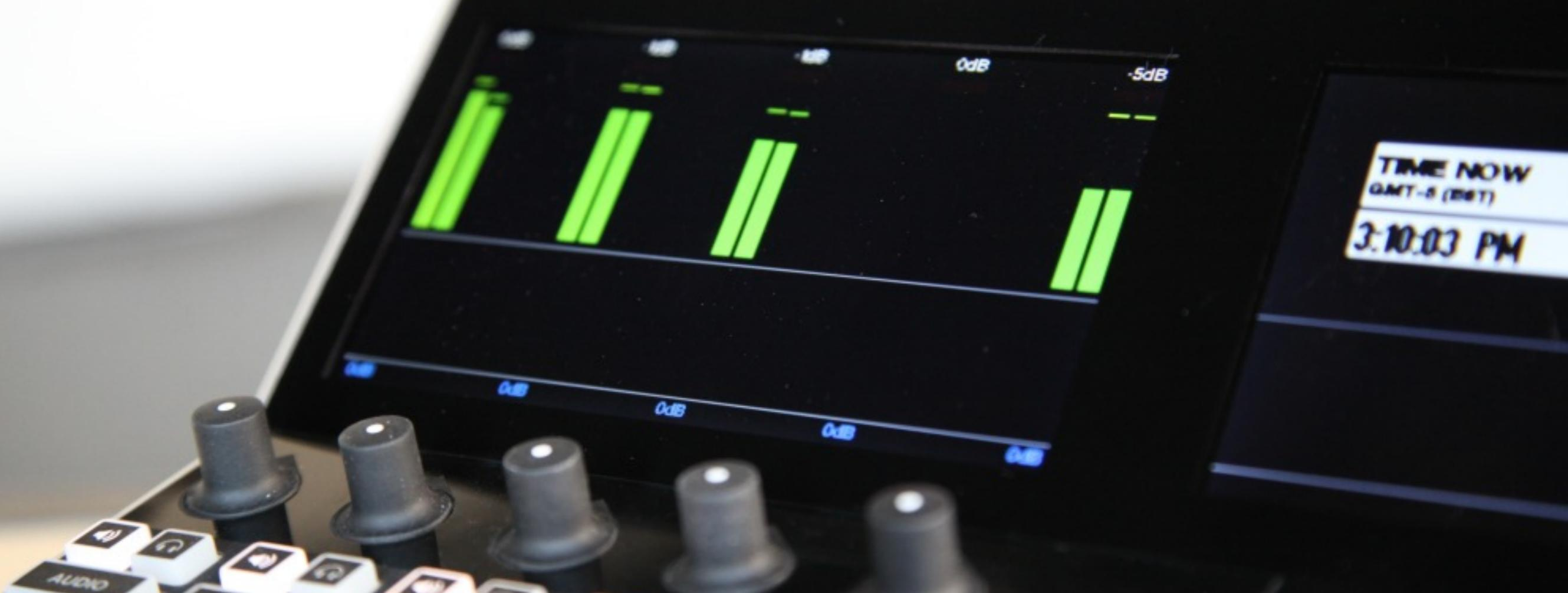
There may be an audio source that you need to adjust the gain on. Turn the knob corresponding to that track to adjust this.
