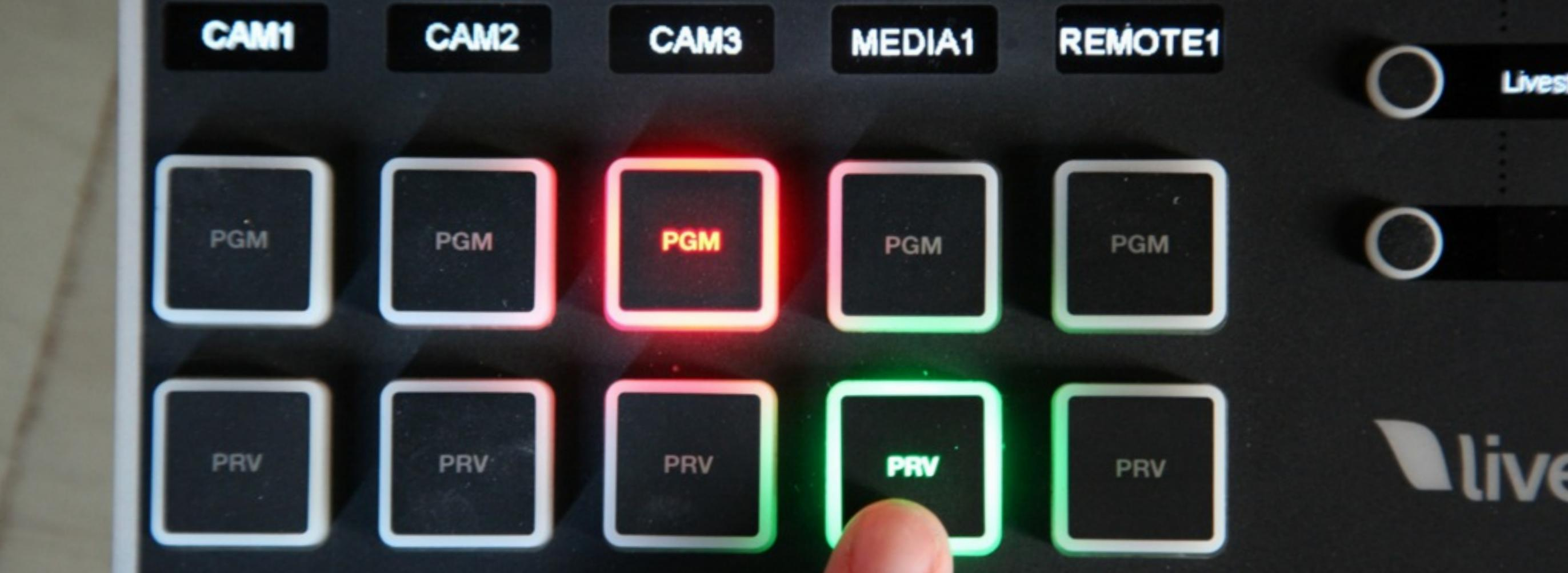
For example, press the **PRV** button corresponding to Media 1.
