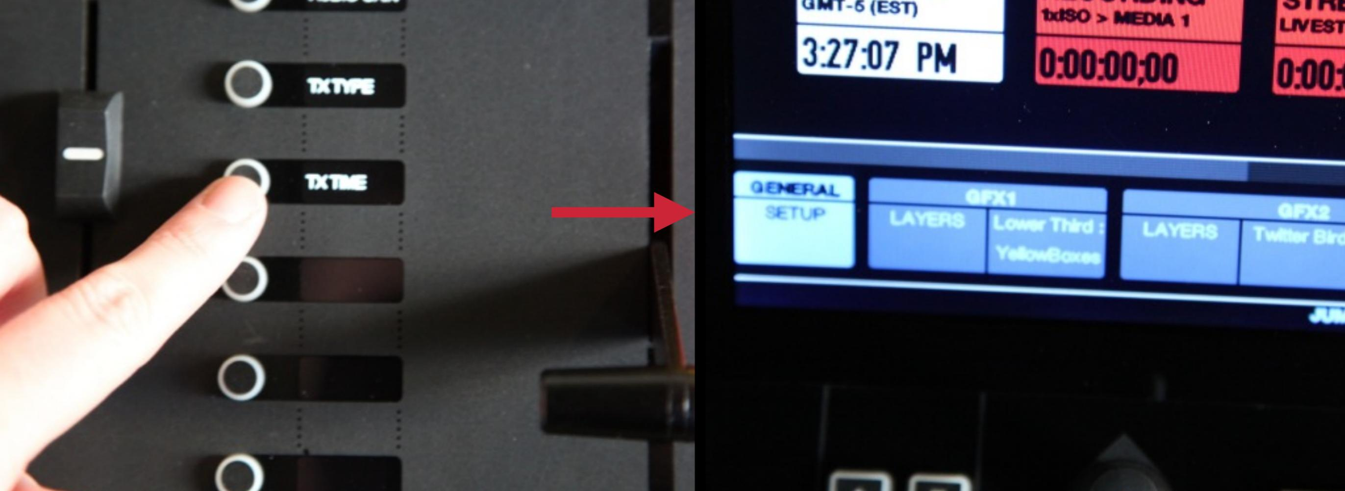
You can return to the main **General Setup** menu display by pressing the currently activated setup menu's **menu button**.
