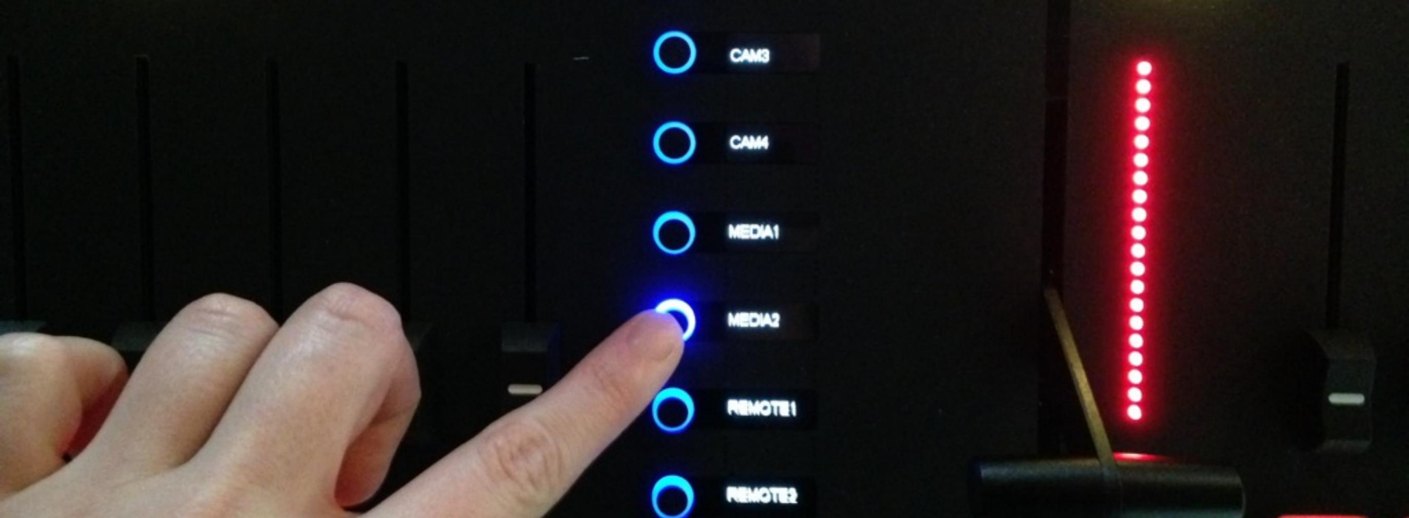
Press any of these buttons to hot change the source that is being used for that AUX. The change will immediately be shown in any graphic or output using that AUX.
