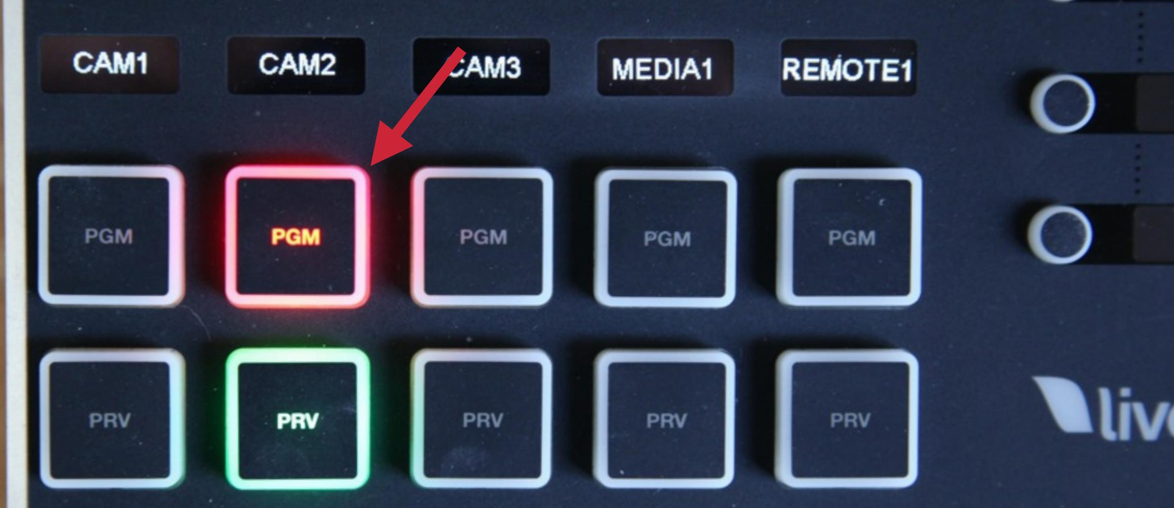
You can also directly put a source into Program without previewing it. To do so, press the '**PGM**' button that corresponds to it.
