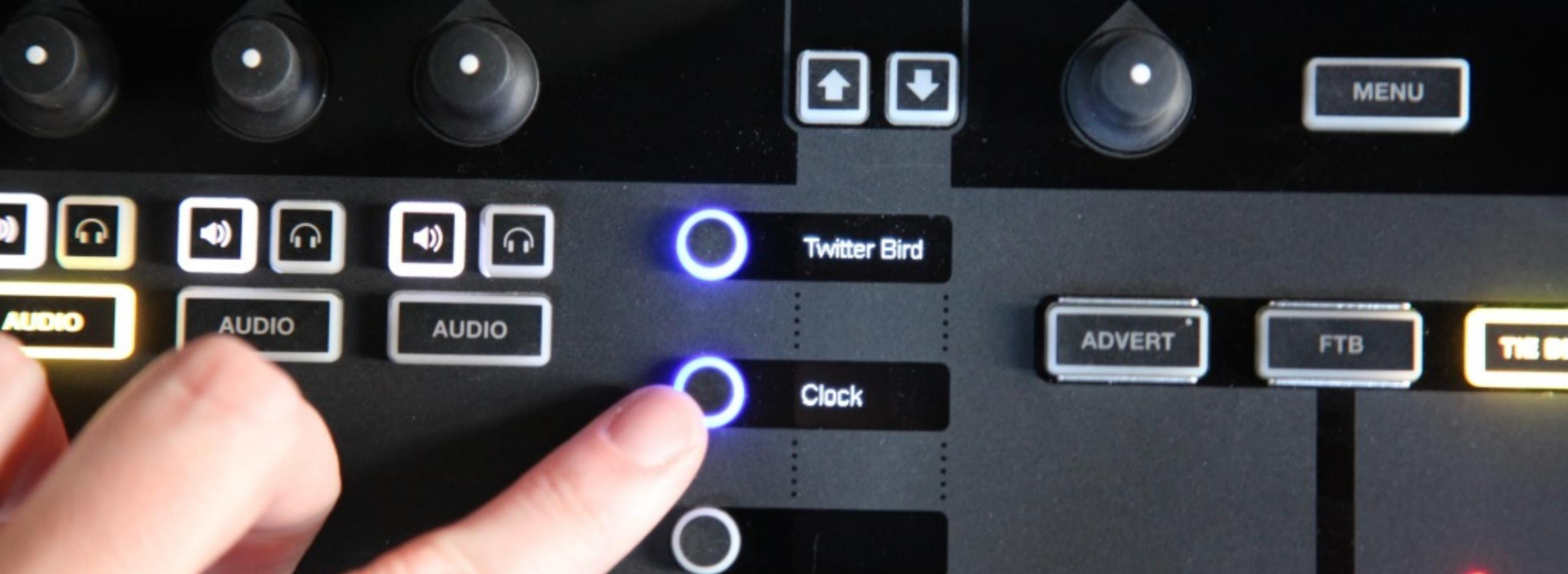
The buttons that are lit up indicate which layers in that GFX channel are visible when in Preview or Program. Pressing the respective button will turn visibility on or off.
