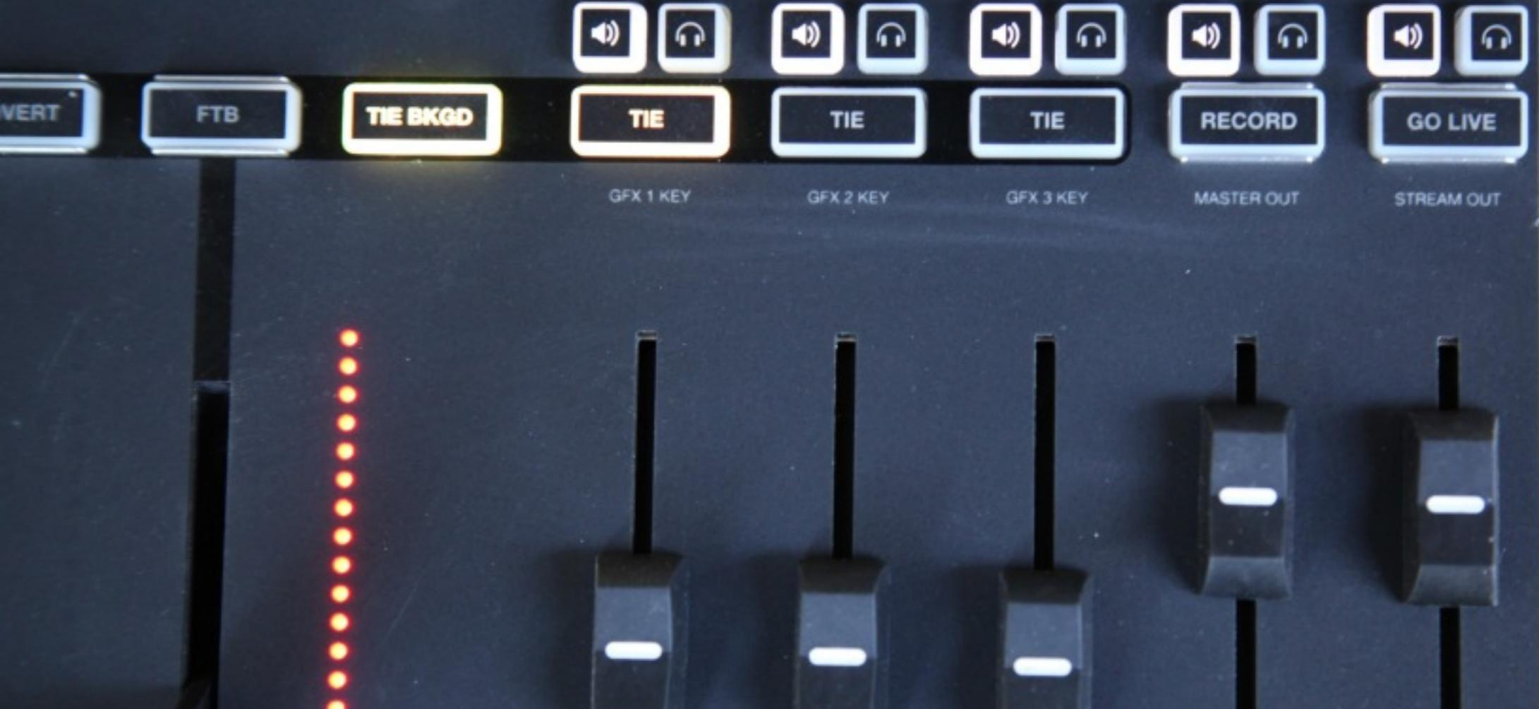
Under the right monitor are controls that adjust the audio levels for the corresponding graphics overlays, Program record, and Program stream.
