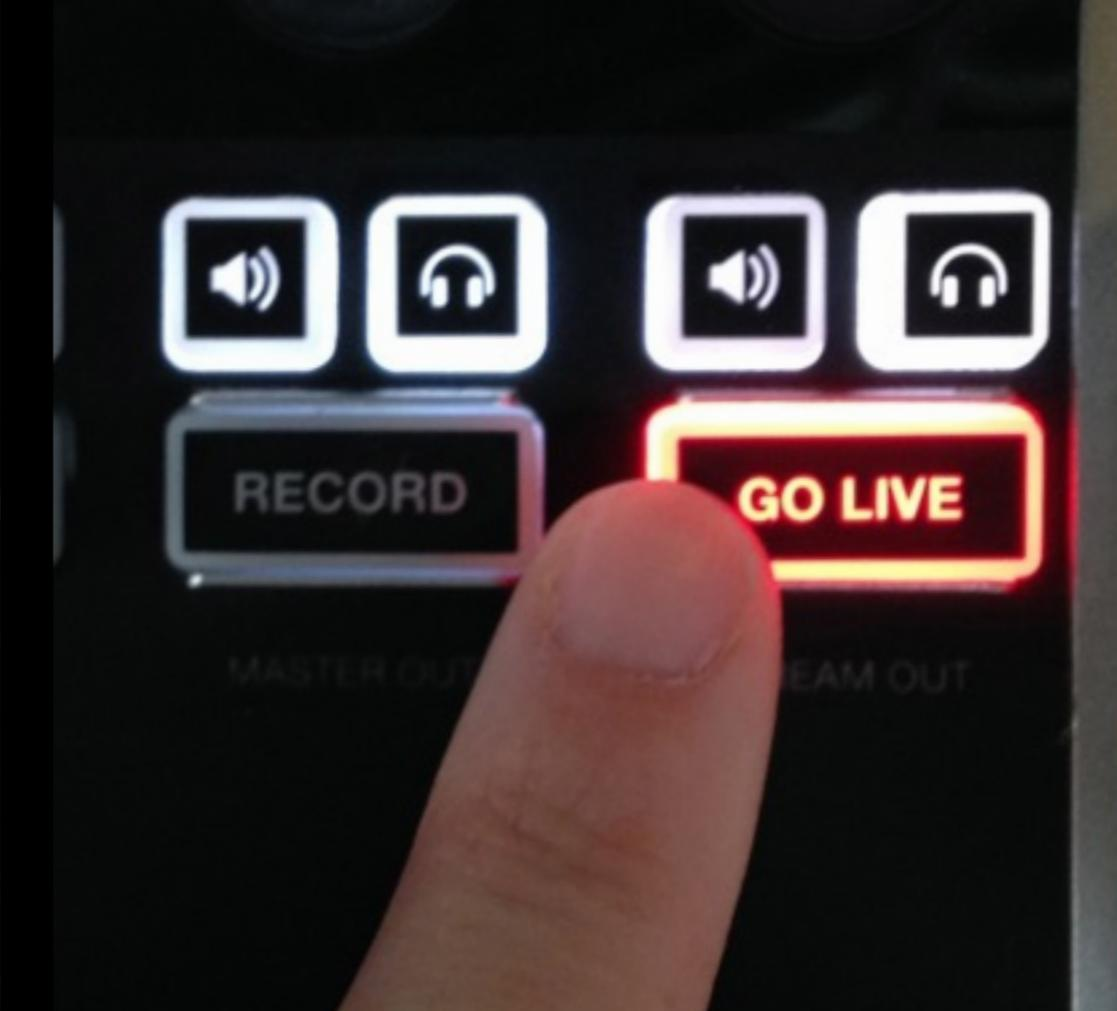
When you are ready to stop broadcasting, you can press either 'Streaming' in Livestream Studio or 'Go Live' on Studio Surface to end the stream.
