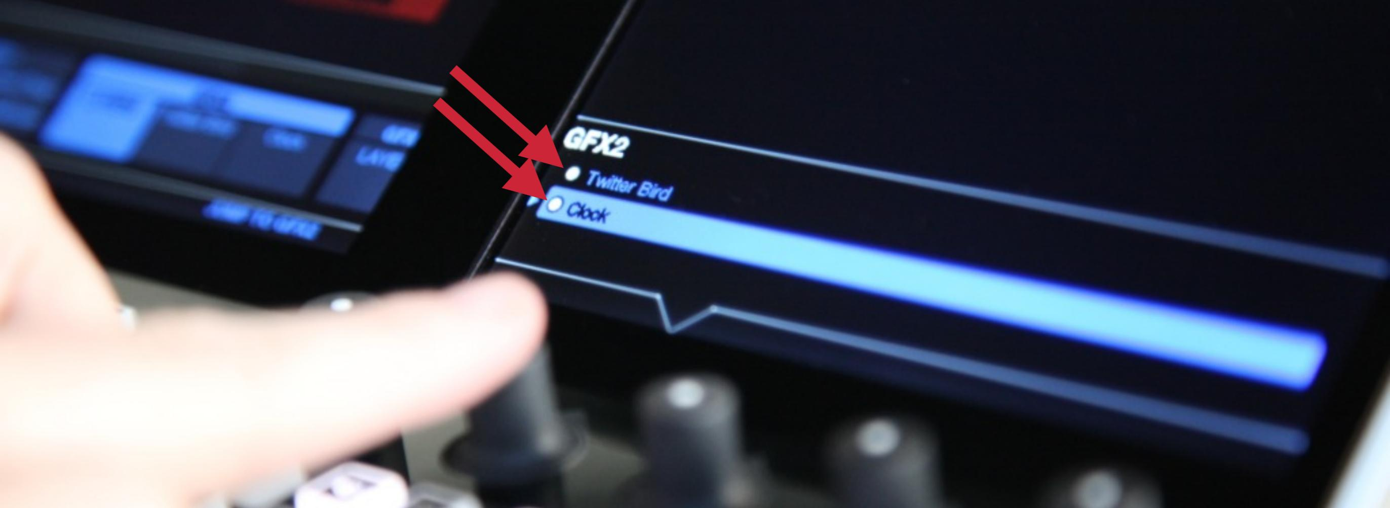
The **white dots** indicate a layer that will be visible when that graphics overlay channel is in Preview or pushed to Program.
