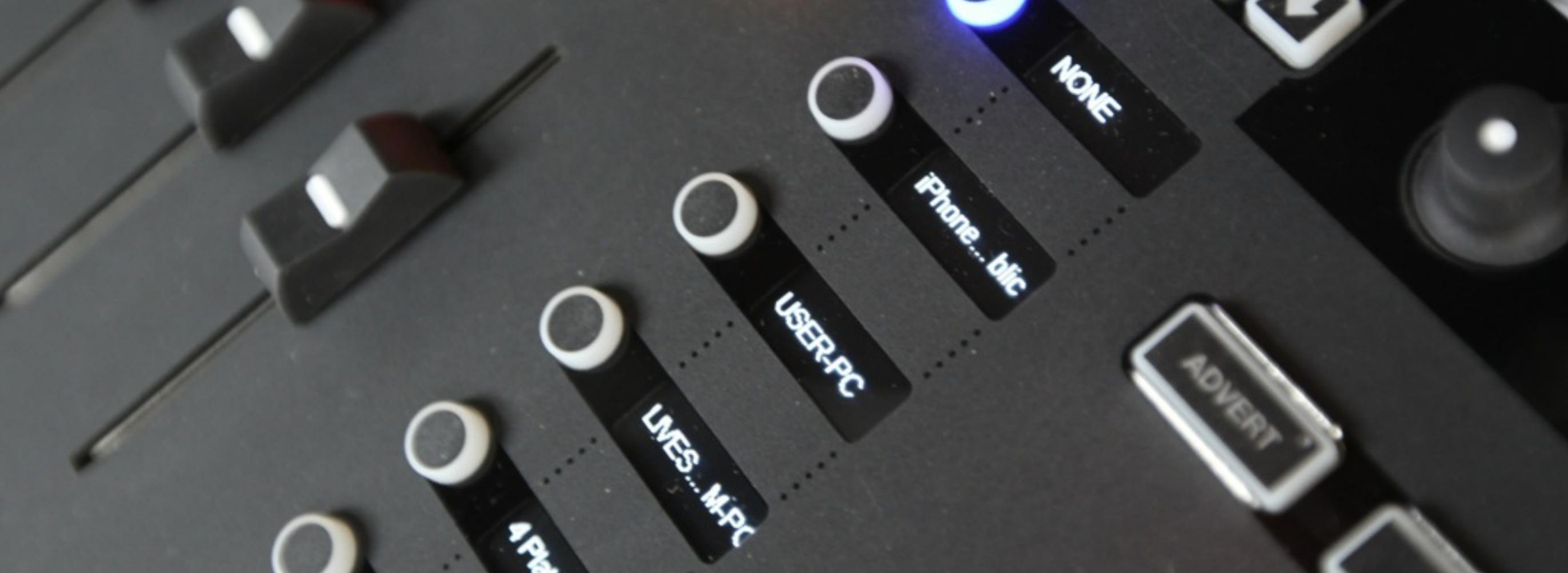
When selecting from either remote camera module, the **menu buttons** will display each remote source that is available to you in Livestream Studio.
