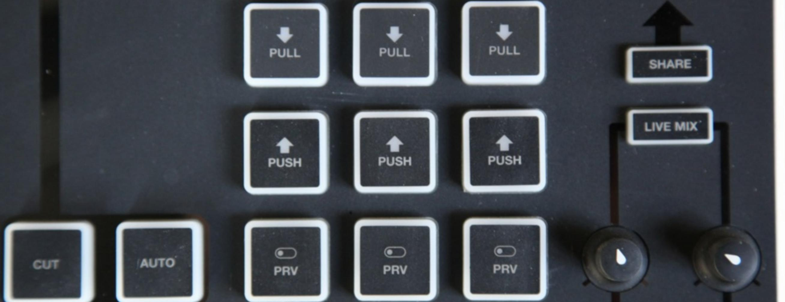
Just to the left of the headphone jacks are the '**PRV**,' '**PUSH**,' and '**PULL**' controls for your 3 graphics overlay channels.
