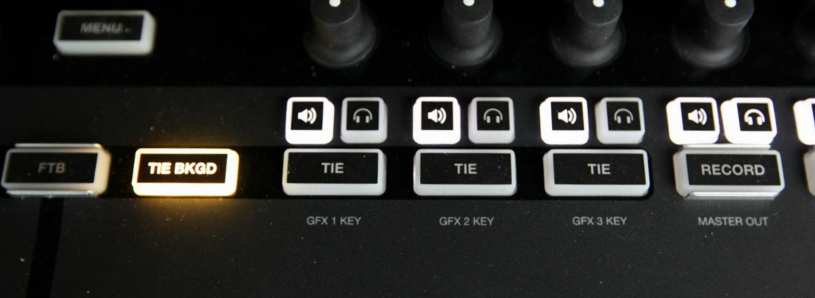
You may need to switch a video source and a graphics overlay simultaneously. This is where the **'TIE BKGD'** and **'TIE'** buttons come in.
