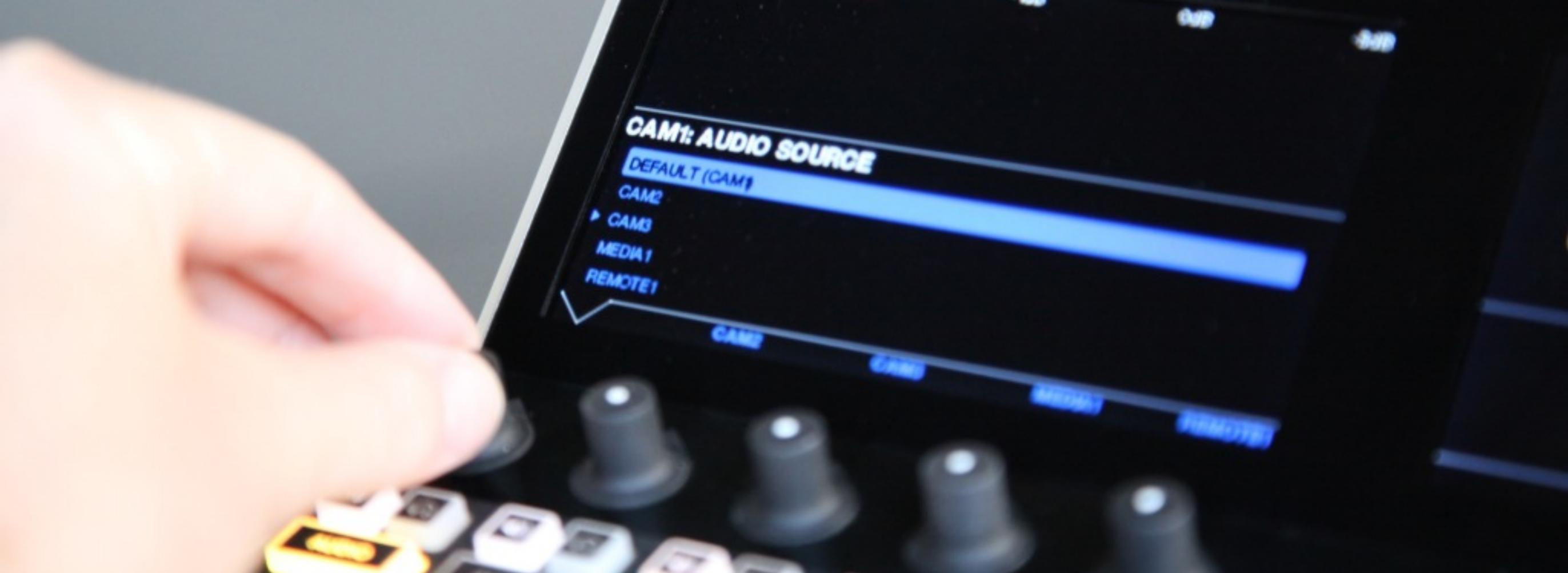
You can revert audio linking by going back to the audio source menu for that video source and scrolling up to the default setting of using its own audio.
