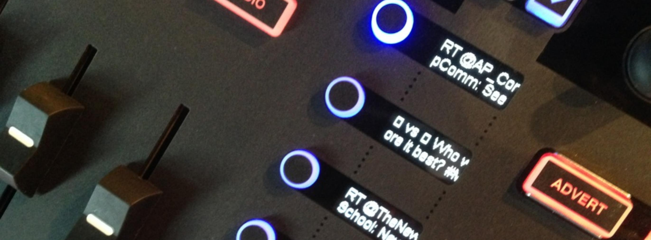
After selecting a layer, the **menu buttons** will display the rows of data available in that layer, such as a manually built row, data from a spreadsheet, or tweets.
