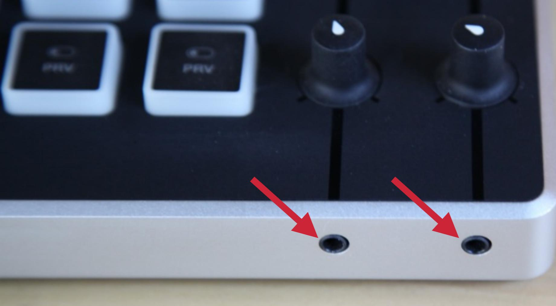
First, to be able to hear your audio sources, plug headphones into either of the two **jacks** on the lower right corner of Studio Surface.
