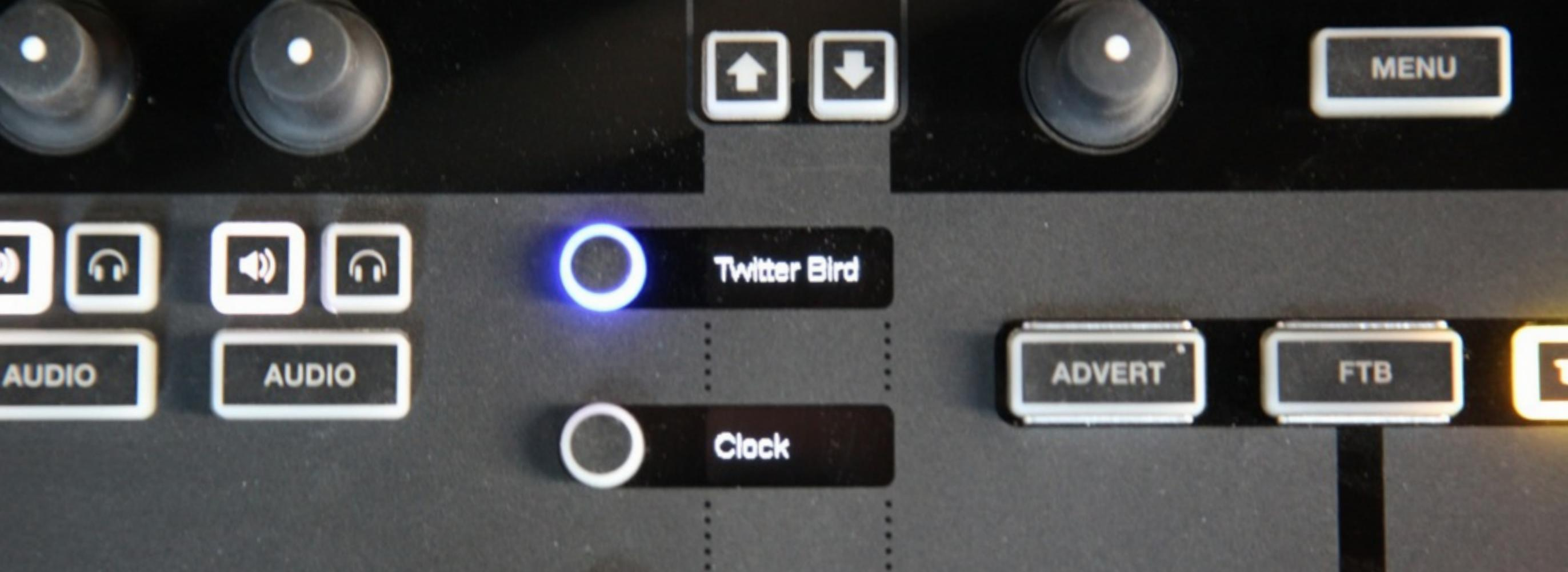
Selecting '**LAYERS**' will show the layers created within that graphics channel on the **menu buttons**. (The two **pagination buttons** above will allow you to scroll to further layers.)
