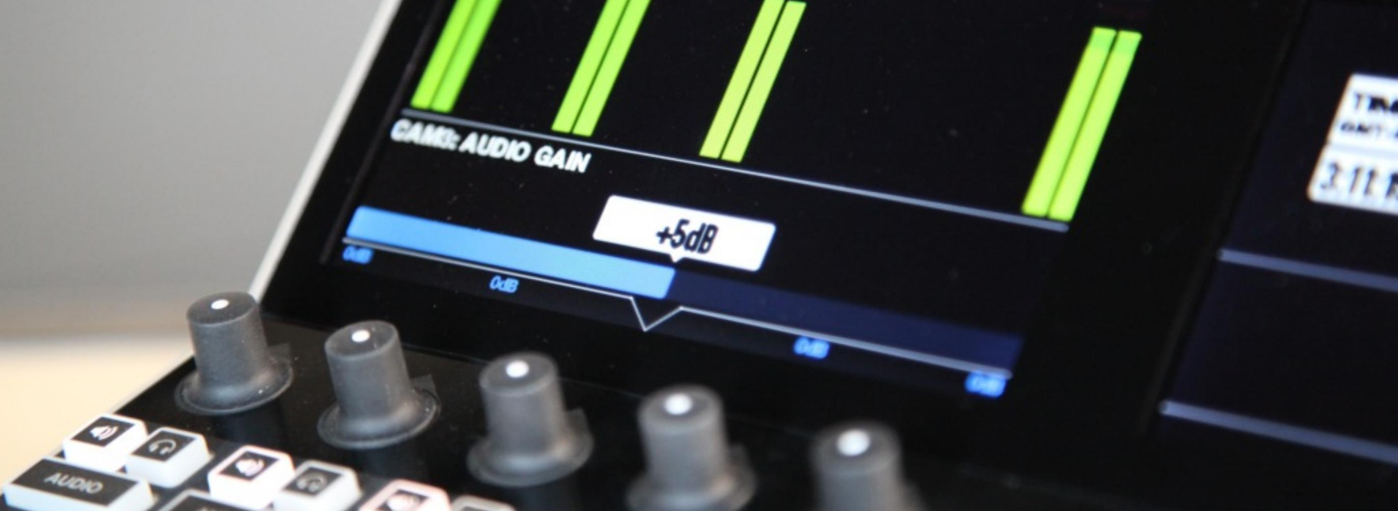
A **gain meter** will immediately appear as you adjust the audio source's gain level. Press down the knob when you have reached the desired level.
