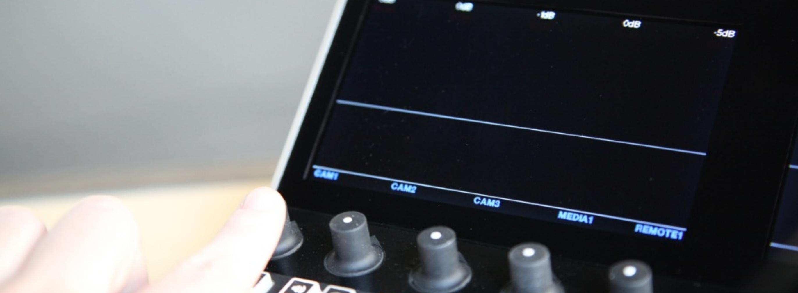
You can change any of these input sources' track assignments directly from Studio Surface. Press down the knob corresponding to the source you want to change.
