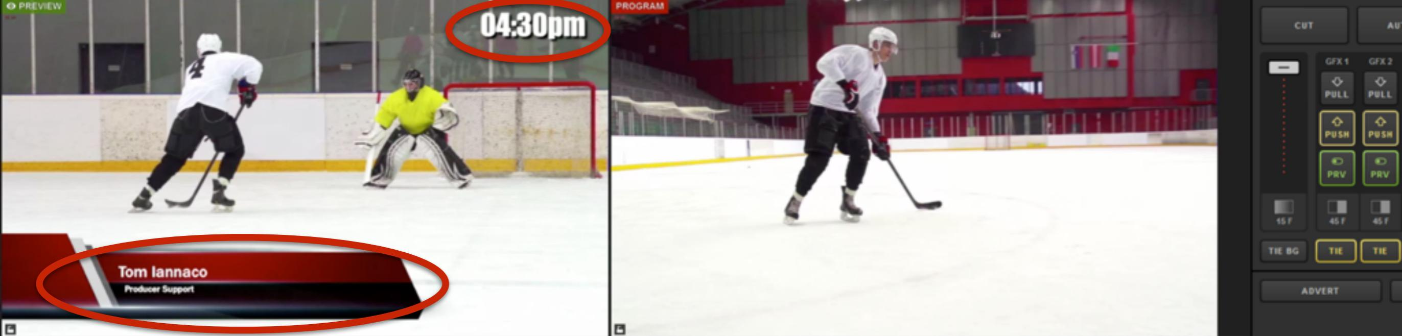
In this example, GFX 1 has a lower-third graphic, and GFX 2 is a clock. Use a transition control to bring both into Program.
