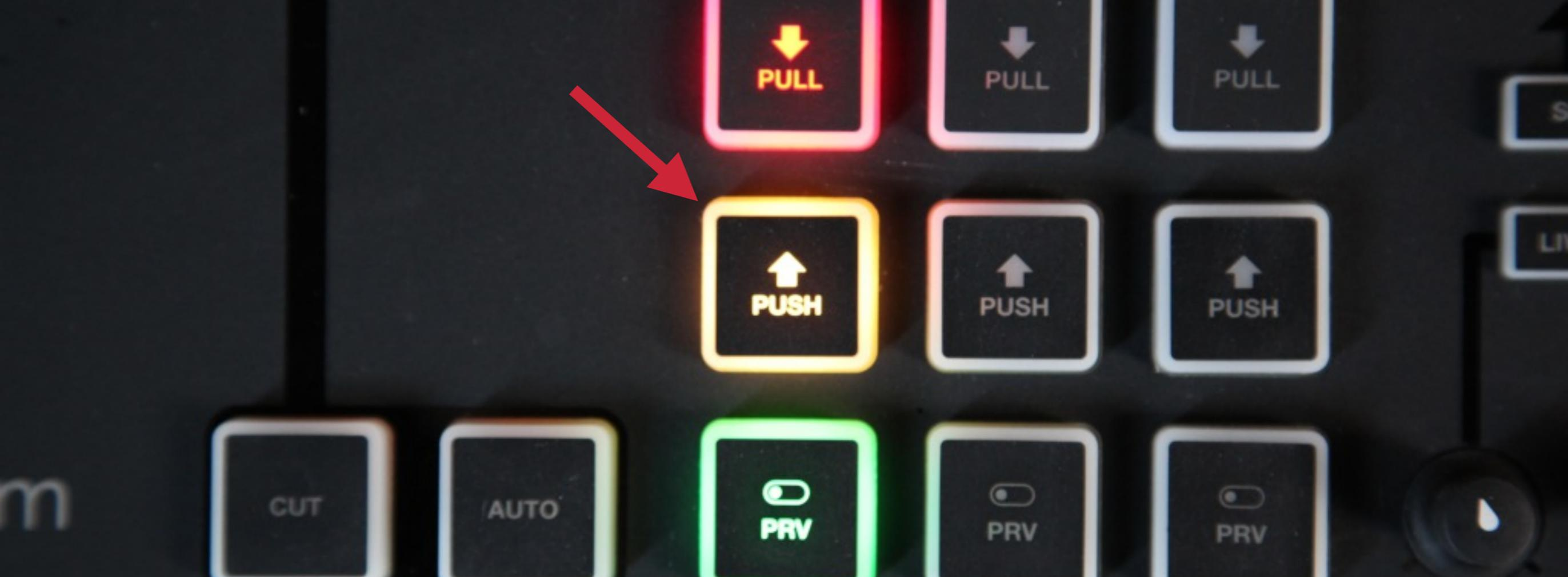
When that change has been made to your active graphics channel, the '**PUSH**' button will begin blinking again. Press it to transition the change into Program.
