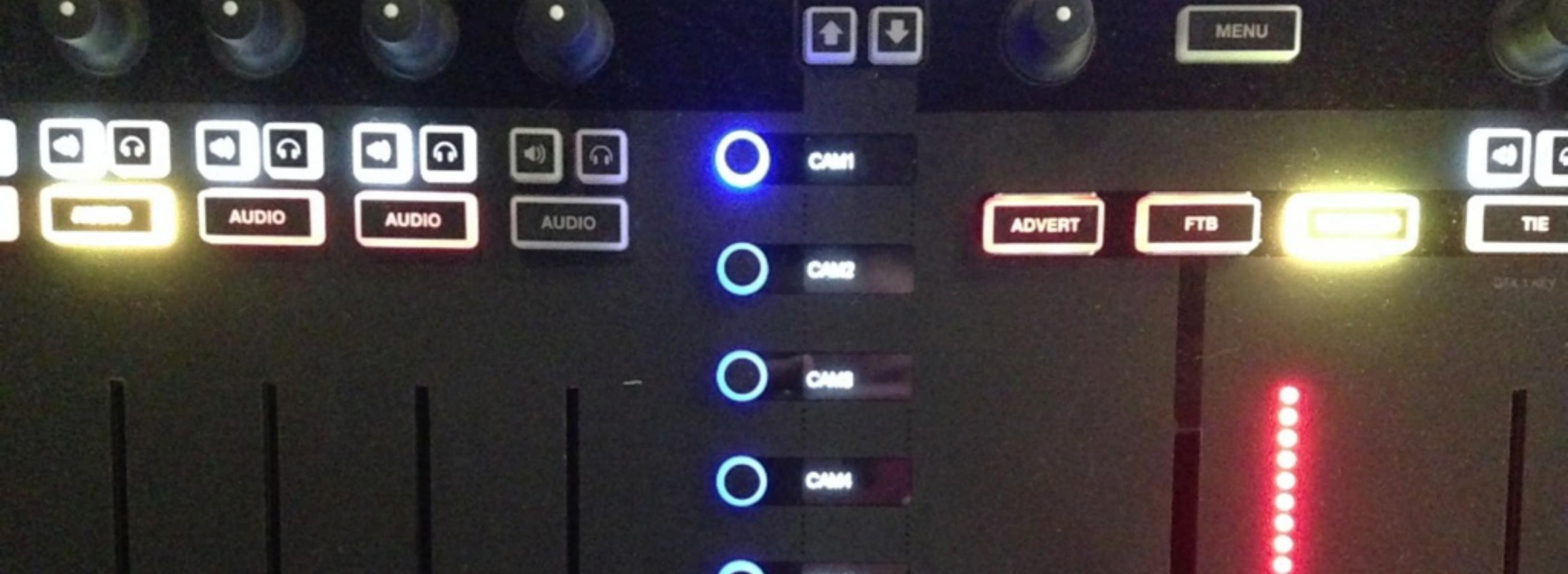
Navigating to an auxiliary menu on Studio Surface will show the same camera sources, media sources and remote cameras in the menu buttons.
