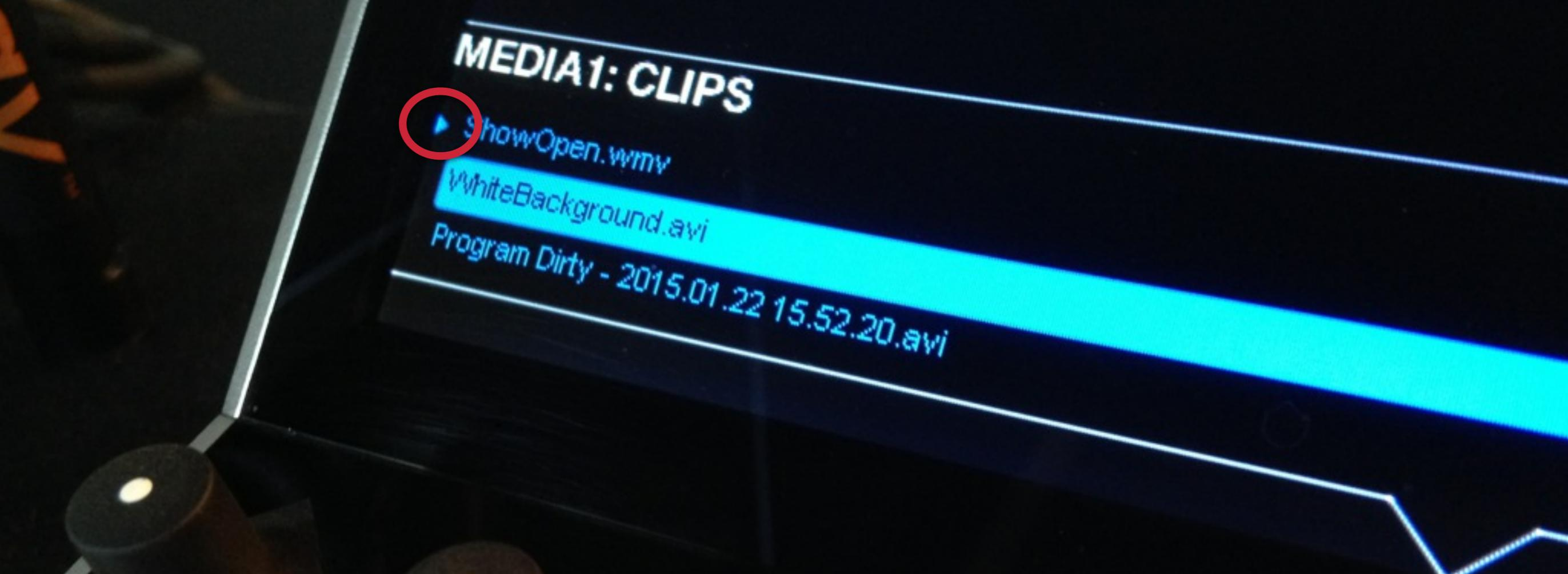
The arrow on the left indicates which clip is currently queued up. Turn and press in the knob to select a different clip.
