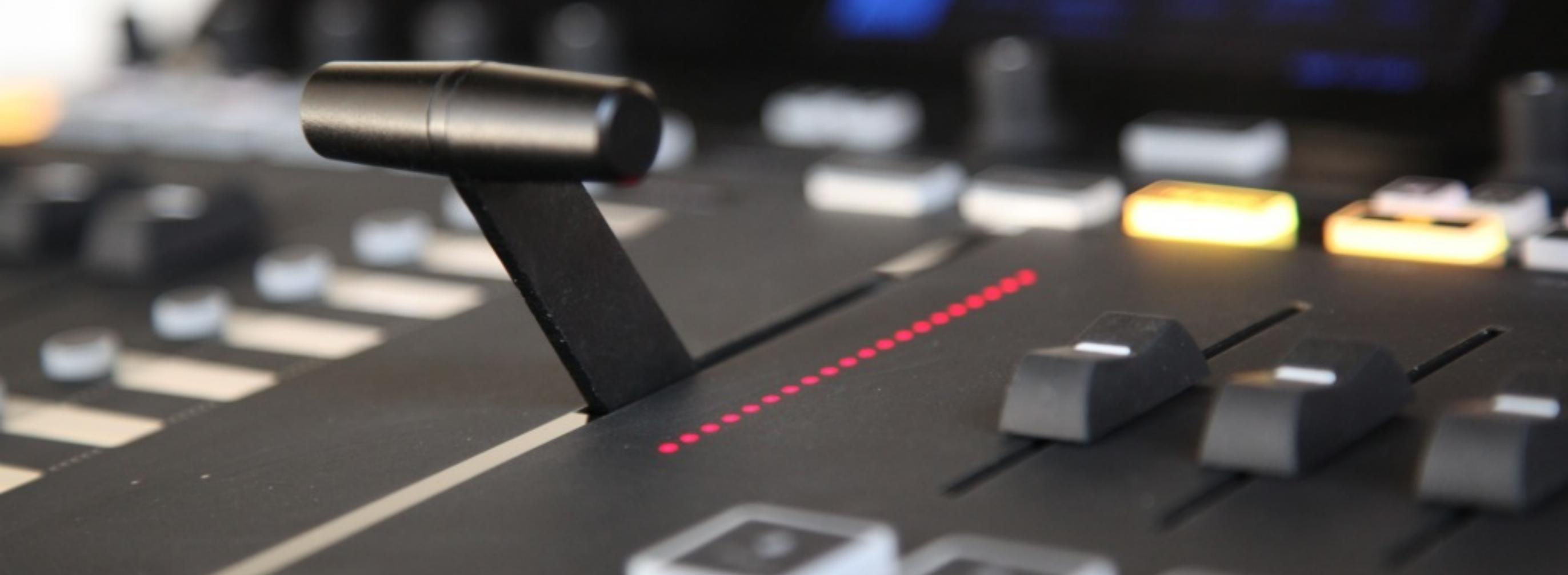
Above the '**Cut**' and '**Auto**' buttons is the **T Bar**, which allows you to do a manual transition between Preview and Program in Livestream Studio.
