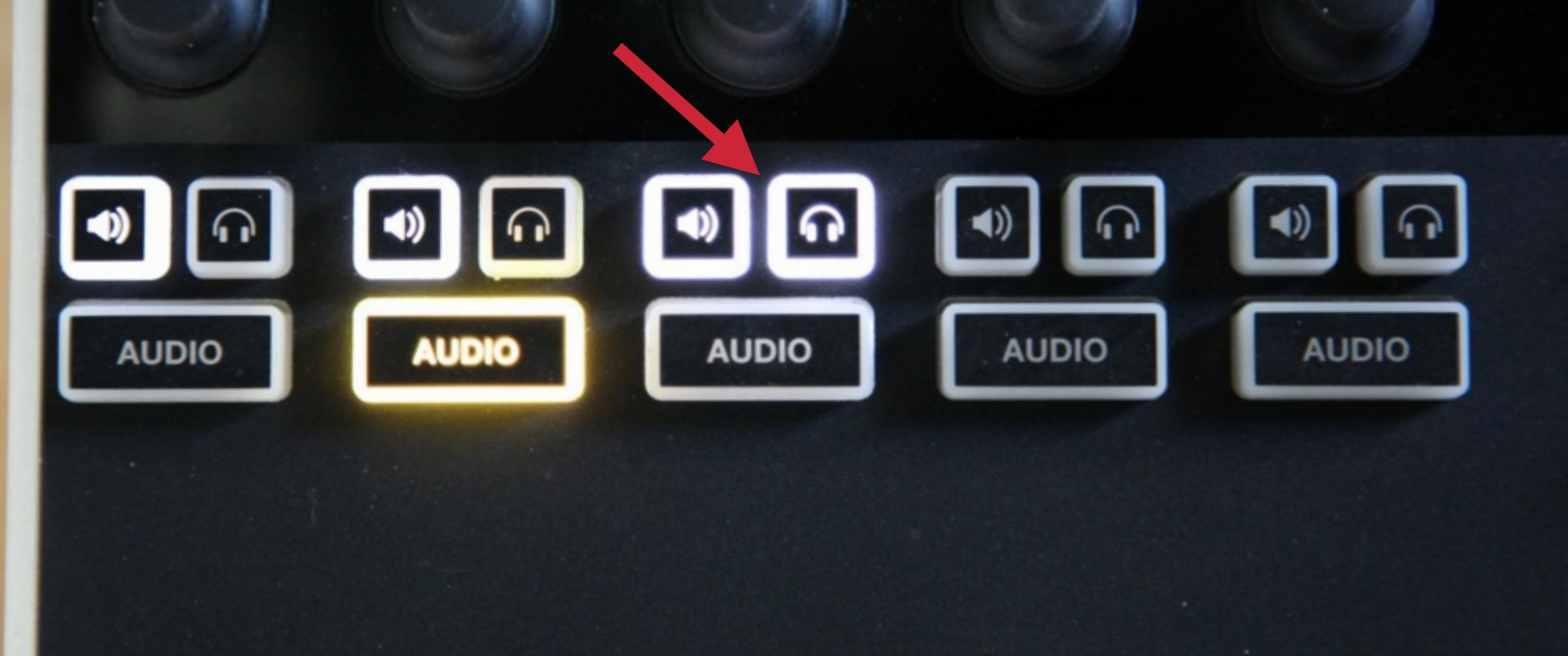
You can use these buttons to isolate each audio source before going live and adjust their levels as needed.
