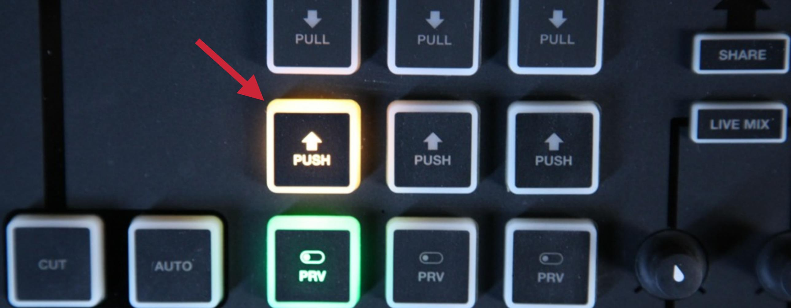
When you are ready to transition the visible layer(s) from that graphics overlay into Program, press the flashing **PUSH** button.
