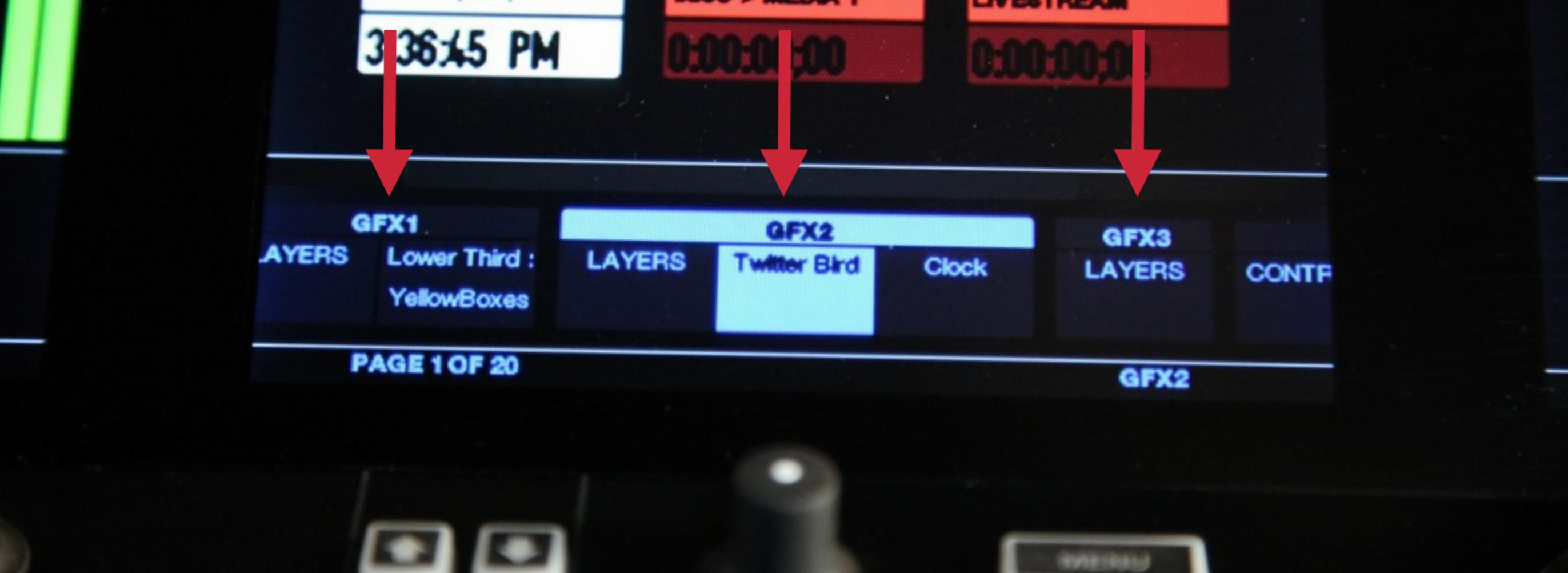
The layers menu and the ability to change data are available for all 3 graphics overlay channels. Use the knob to scroll to the other channels.
