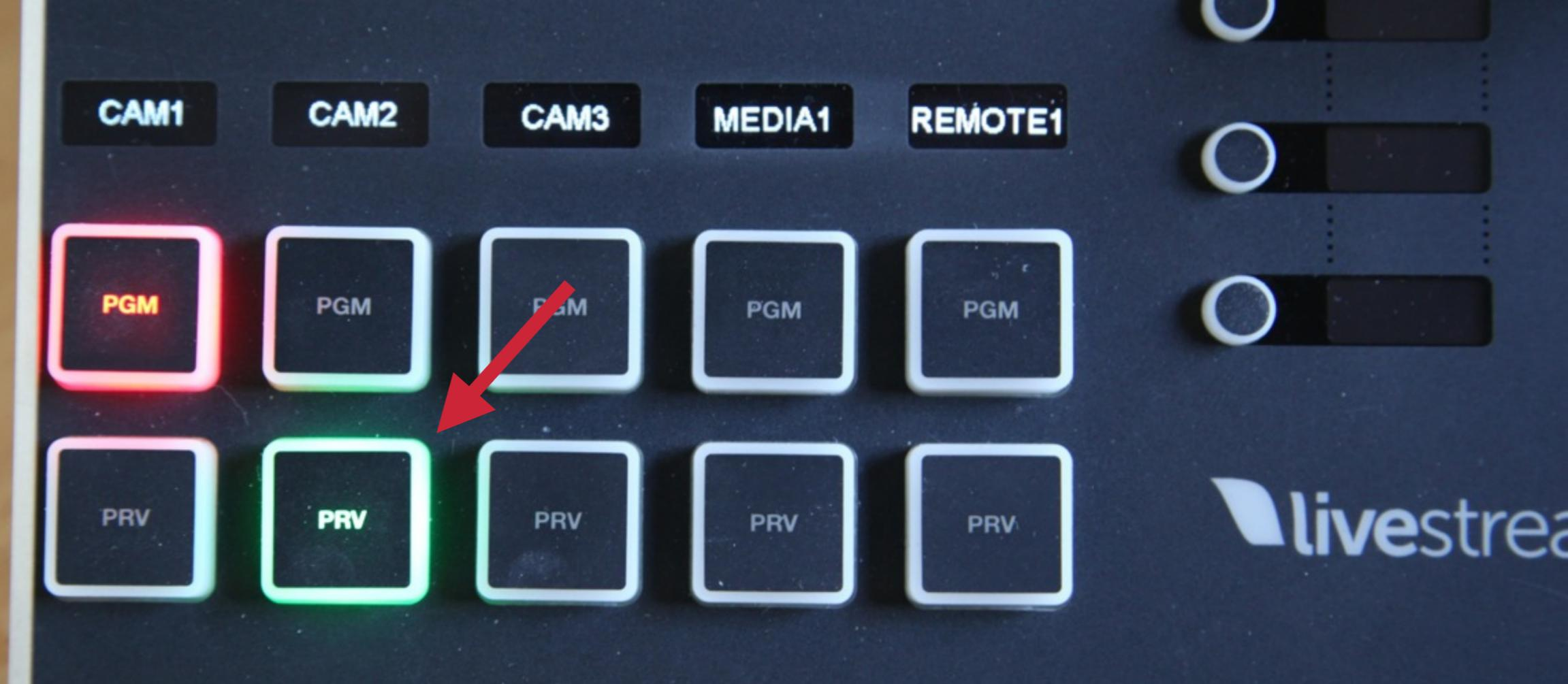
To put a source into Preview, press the green '**PRV**' on the track that corresponds to that input source.
