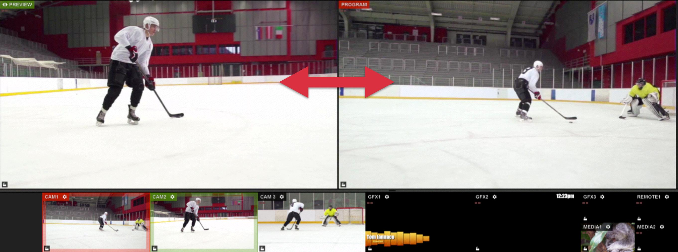
A typical multi-camera production involves putting a source into Preview and then switching it with the source in Program using a transition control.
