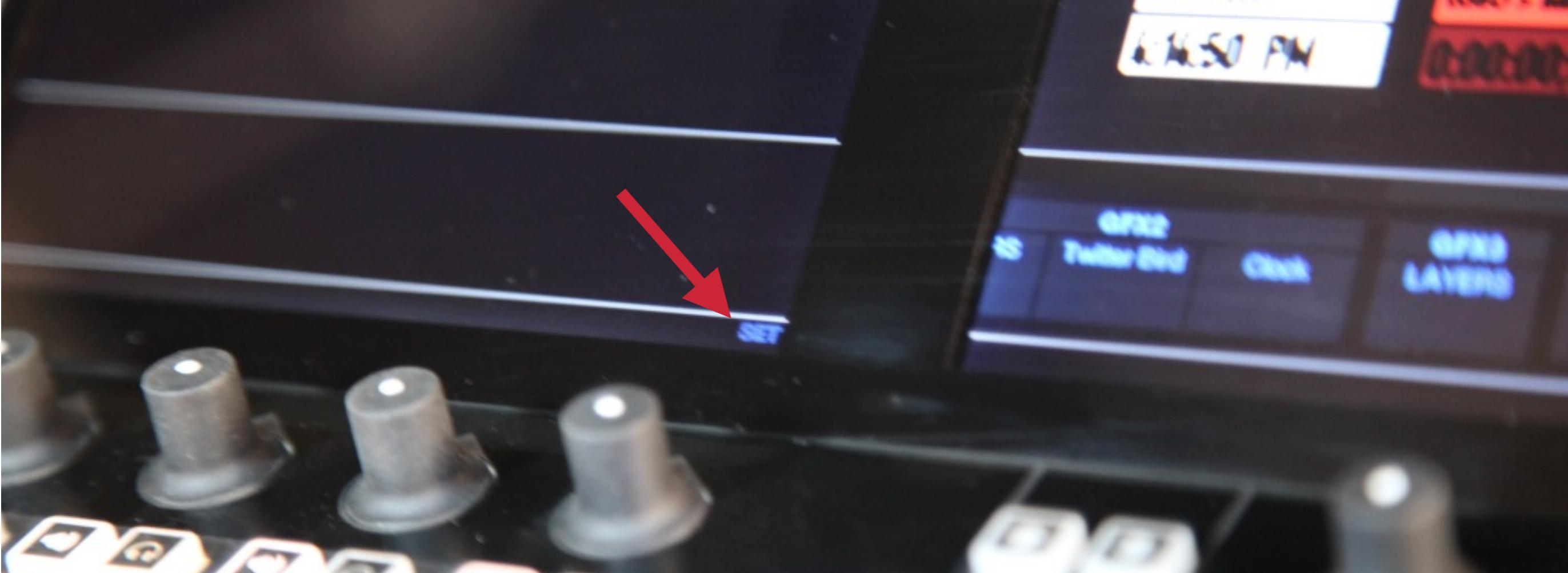
The track that the camera is assigned to should start blinking '**SET**' at the bottom of the monitor. Press in the corresponding knob.
