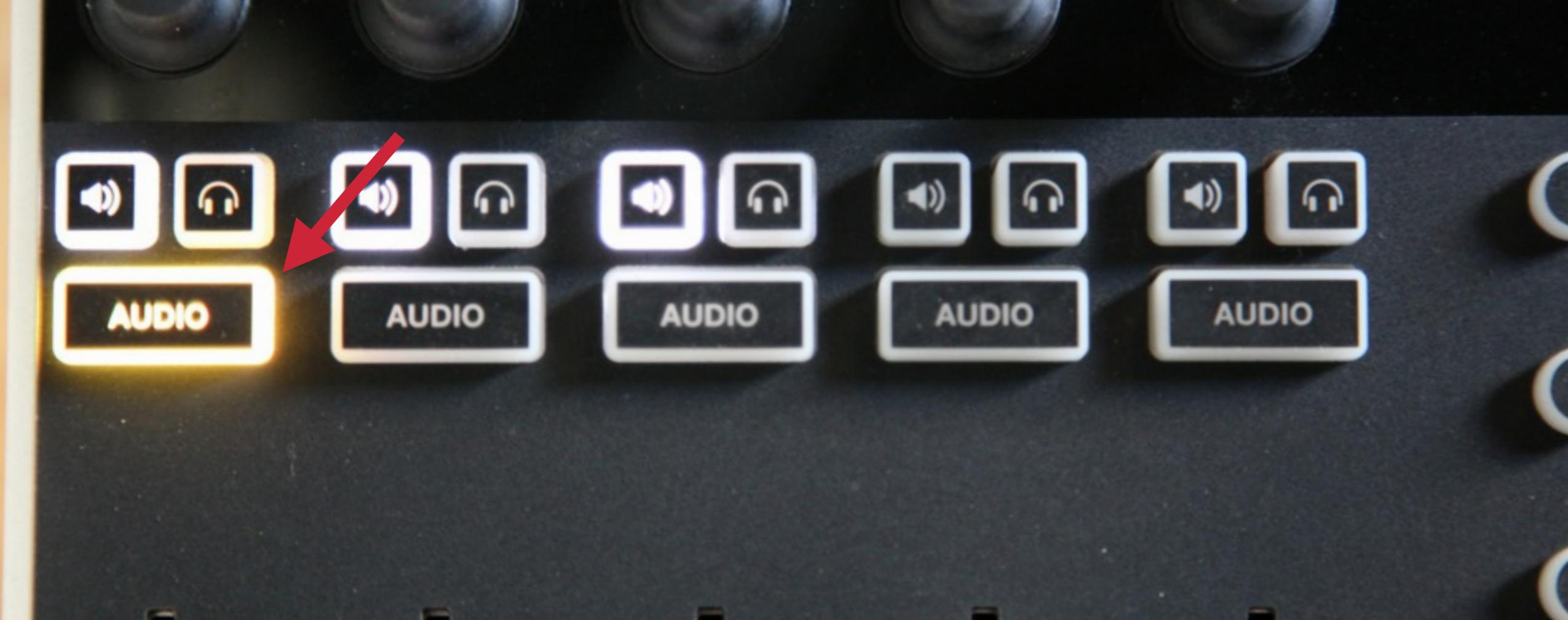
When switching between your video sources, you may notice different audio controls on the left lighting up and turning off during transitions.
