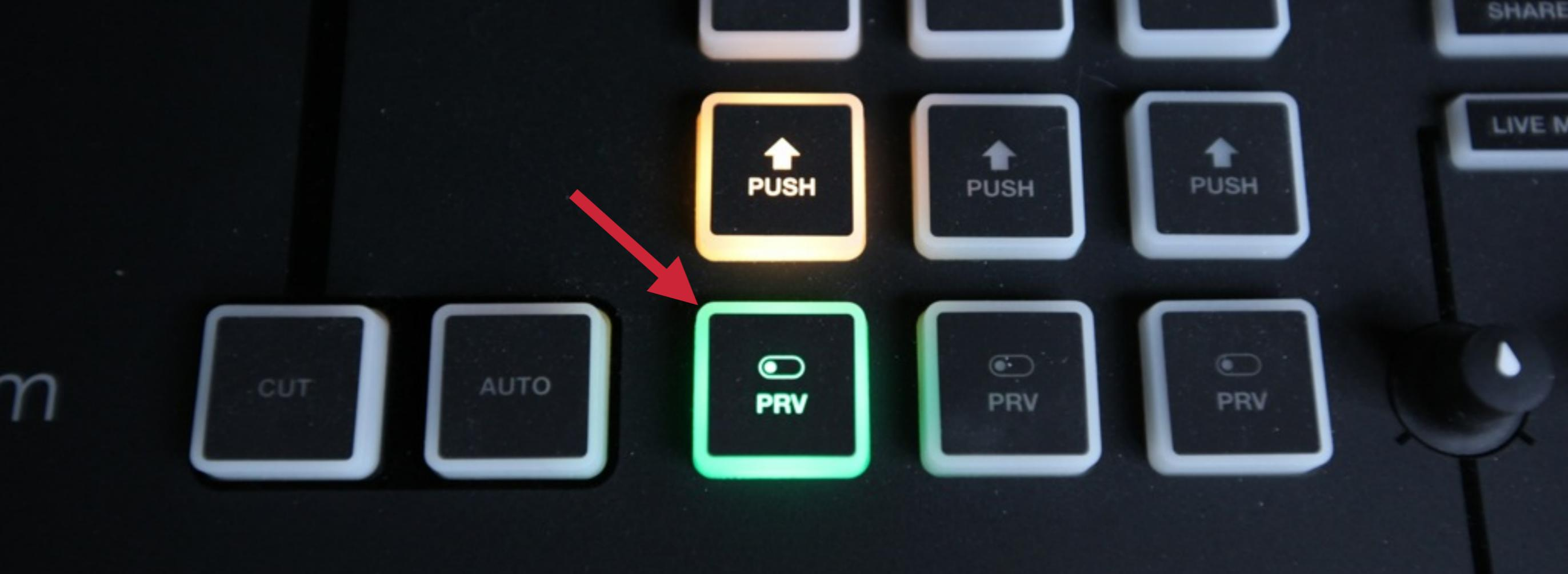
Press the '**PRV**' button for the graphics overlay channel that is tied to your video source.
