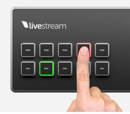
Similarly, to put a source directly into Program, press the corresponding 'PGM' button.
