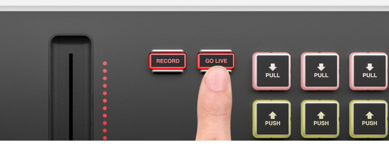
When you first press either button, they will light up red to indicate that they are active. Press the button again to stop the recording or streaming.
