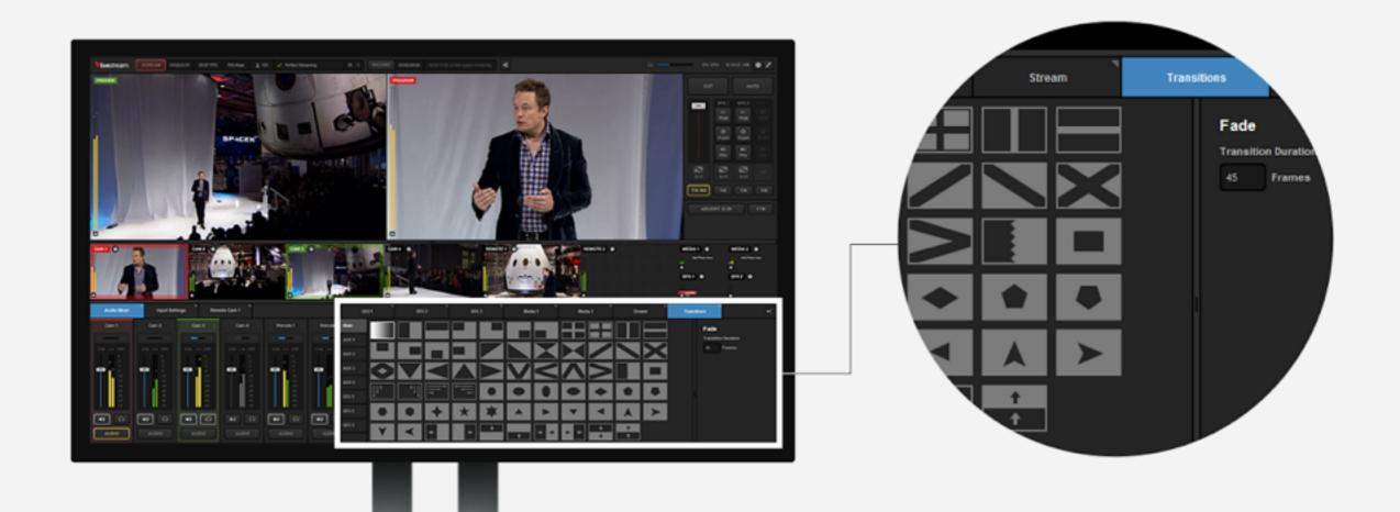
The 'Auto' transition type and speed is determined in Livestream Studio under the 'Transitions' tab.
