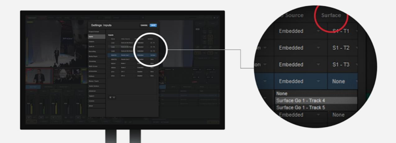
In Livestream Studio settings, navigate to the 'Inputs' menu. Under the 'Surface' column, you will assign five inputs to the five tracks on your Surface Go.
