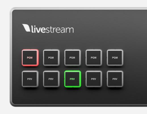
After saving your settings, the Surface Go will indicate which of your assigned sources are in Preview and Program. The track with the lit green 'PRV' button is in Preview. The track that has the lit red 'PGM' button is in Program.
