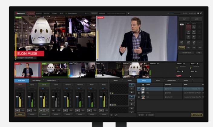
The red 'PULL' button will light up, indicating that the graphics overlay is in Program. Press it to remove the graphic from Program.
