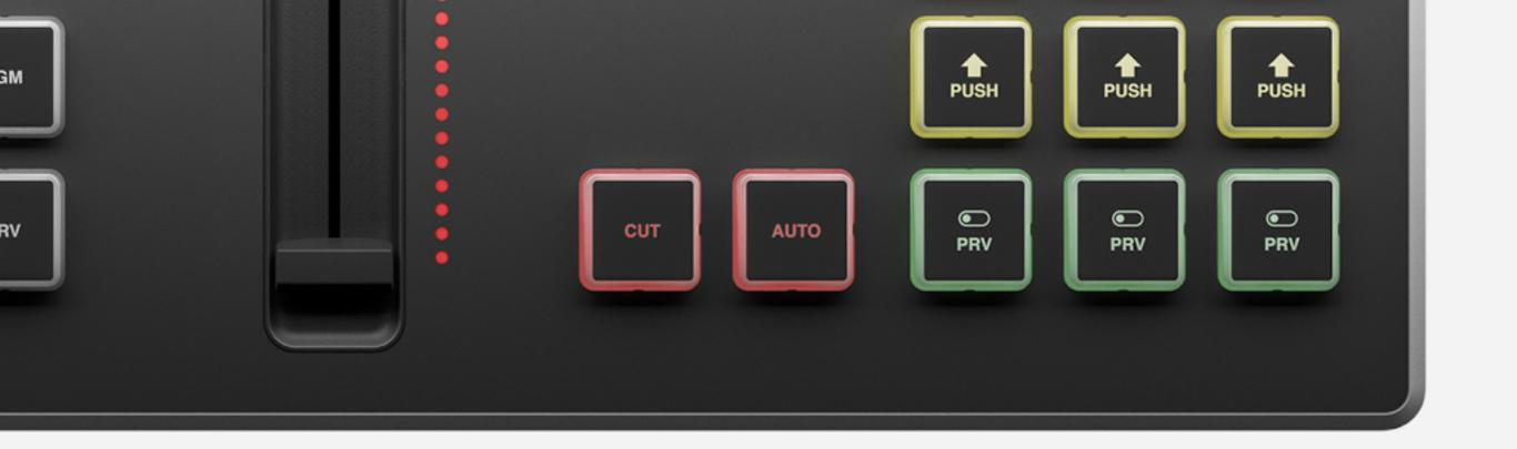
The Surface Go also includes 'Cut' and 'Auto' transition controls for switching sources between Preview and Program.
