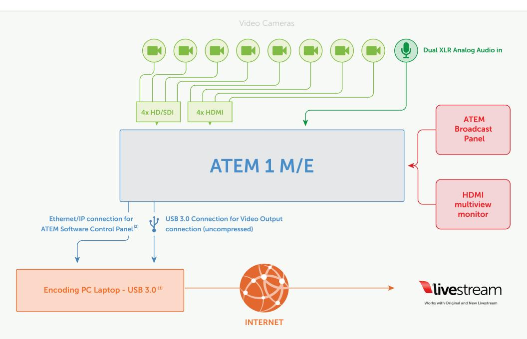
[1] Running Livestream for Producers (New Livestream) or Livestream Procaster (Original Livestream) for live, multi-bitrate encoding from the USB 3.0 ATEM connection
