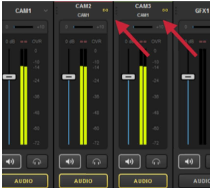
Most producers link Record Out and Stream Out together for consistent Program audio across all output sources. Those two outputs may be unlinked if desired, but they cannot be linked to any other source.
