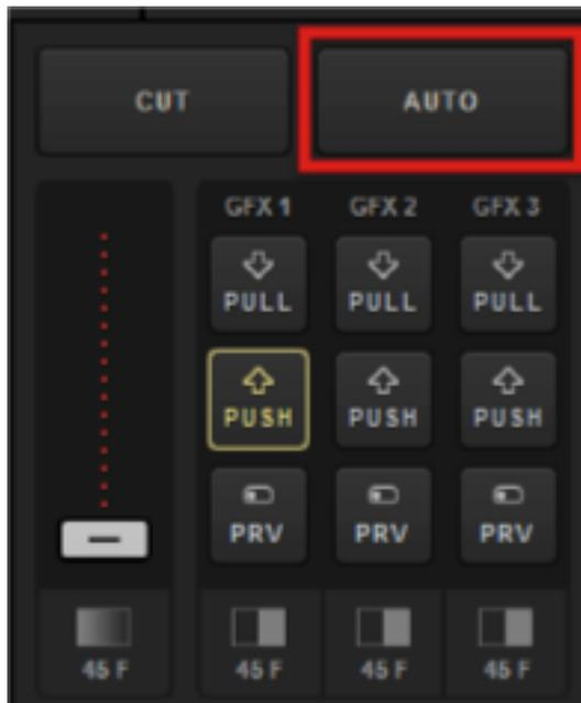
You can always employ a manual transition by clicking and dragging the virtual T Bar below the transition buttons. This allows you to control the speed of that transition.
