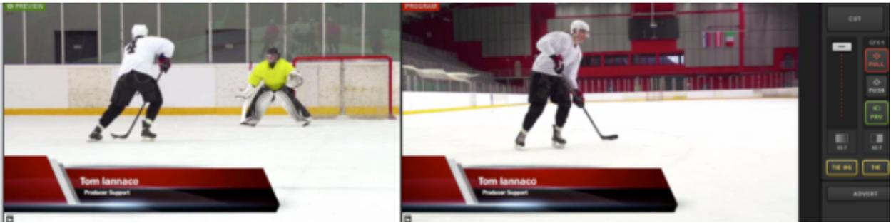
If only the GFX 1 and GFX 2 TIE buttons are lit and both sources are in Preview, then both overlays will switch into Program when transitioning. The video will not change.
