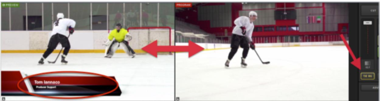
To switch the video source and bring in a graphics overlay at the same time, select TIE BG and the corresponding TIE button for your graphic. Be sure to select the PRV button for the graphics overlay channel that is tied to your video source.
