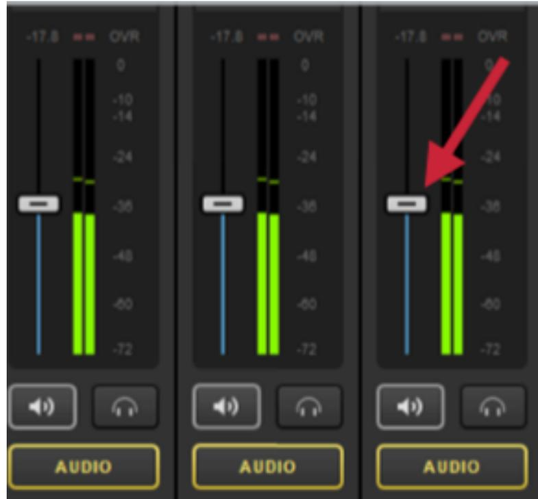
If audio levels are too high, the mixer's OVR meter for any over-modulating source will blink red.
