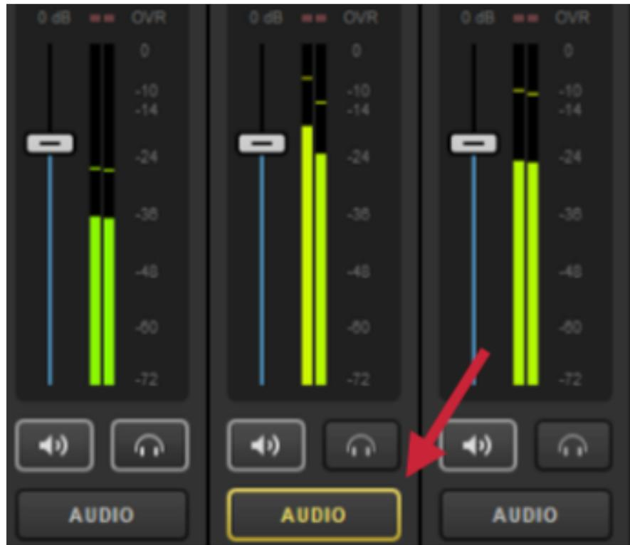
This indicates that the audio source is heard in Program because its corresponding video input is in Program. It is not heard when the video input is not in Program.
