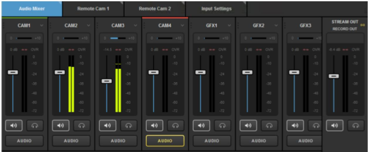
Each input source will have a corresponding audio source that you can monitor and adjust.
