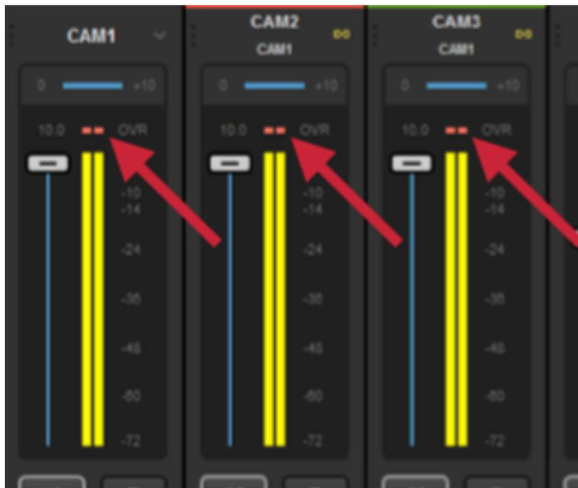
You can also adjust the gain of each source by clicking and dragging the small gain meter above that source's level meter.
