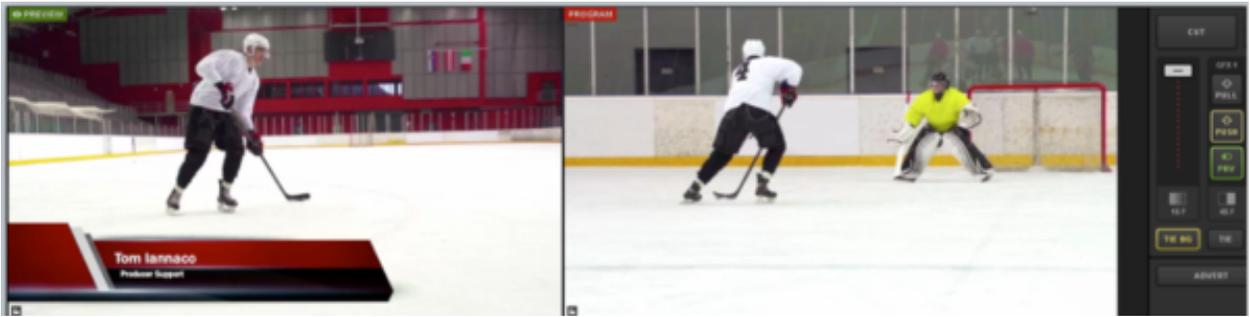
After using a transition control, notice how the video source switched, but GFX 1 remained in Preview because only TIE BG was selected.
