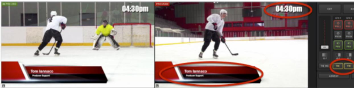
To pull a graphics overlay out of Program simultaneously with a video source, tie the background and the graphics overlay together.
