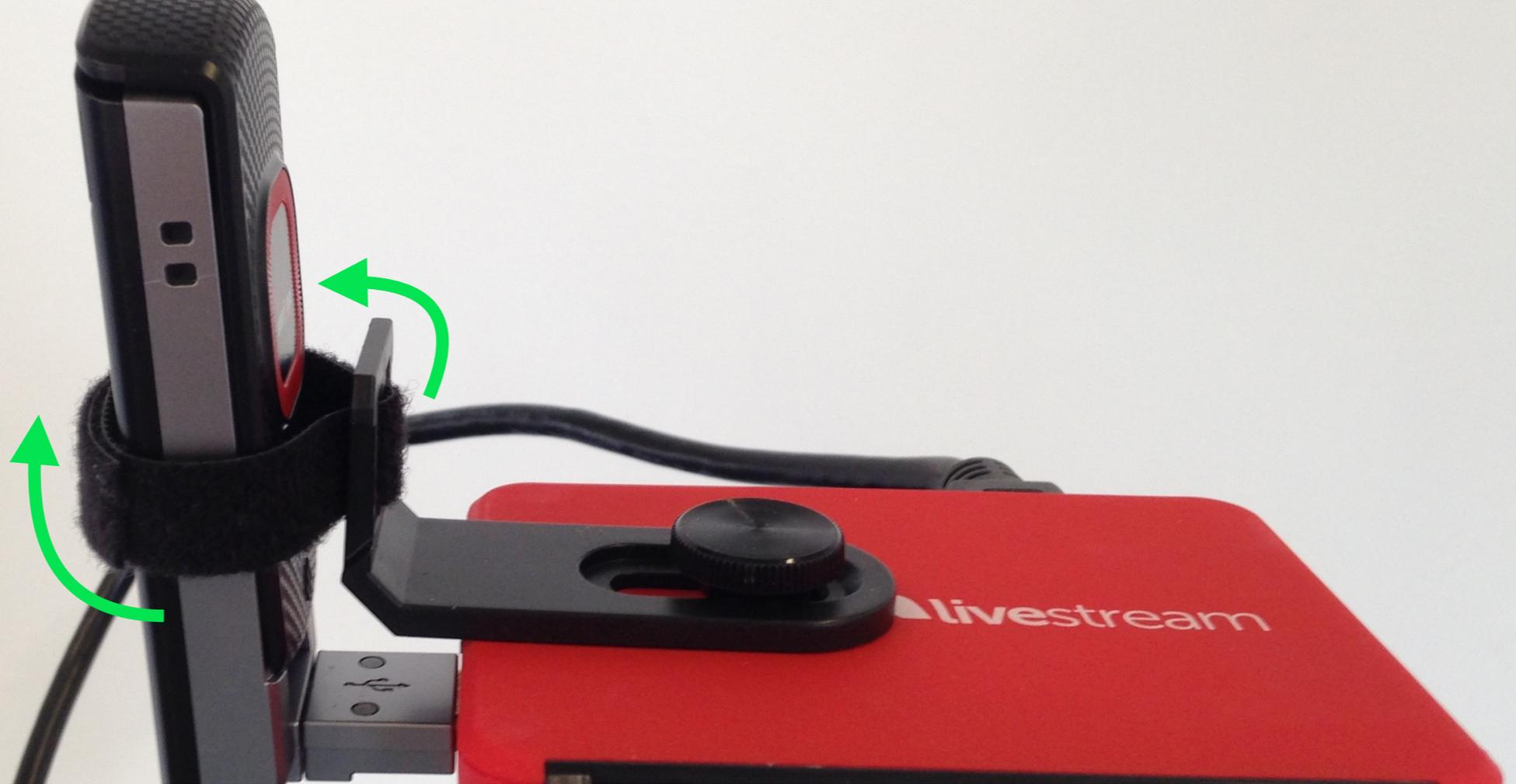
Wrap the Velcro strap around the modem to ensure the modem will stay in place.
