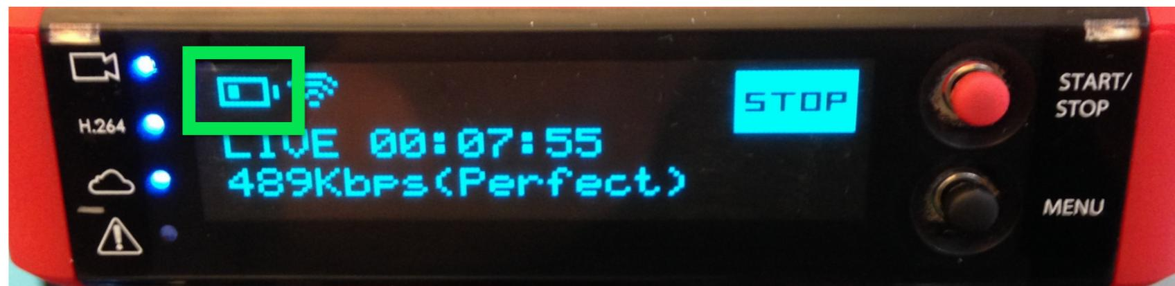
If the Broadcaster Pro is plugged in and the AC adapter is unplugged, the Broadcaster Pro will immediately switch to battery power with no interruptions, and vice versa.
