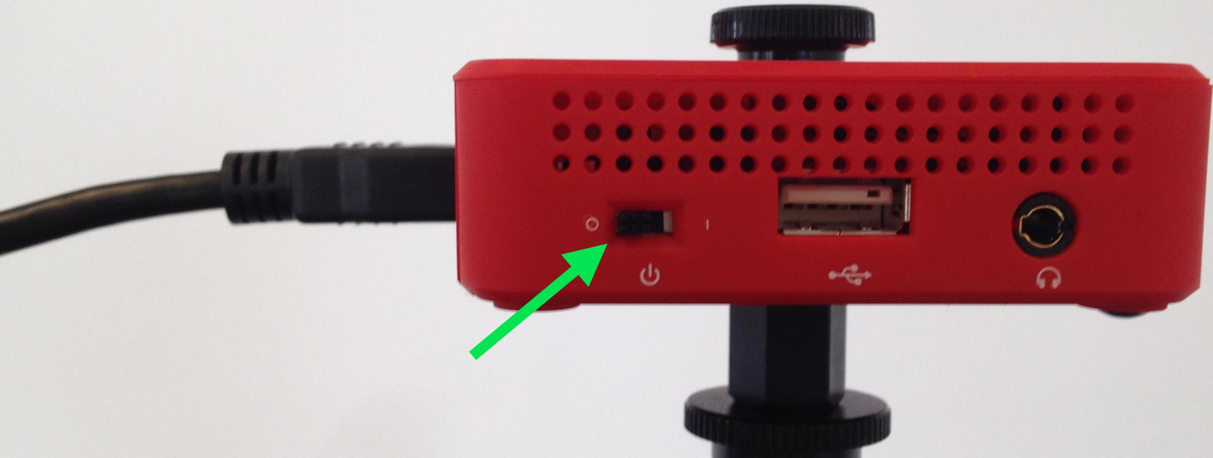
Always turn the camera power on before turning the Broadcastcaster Pro on using the power switch on the side.
