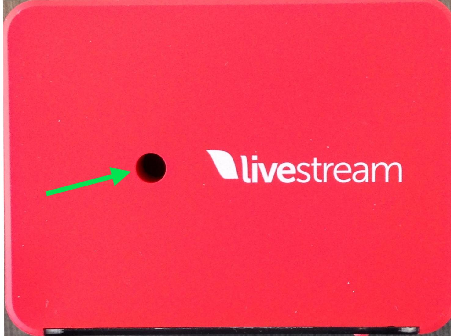
The hole for the thumb screw used with the shoe mount is visible from both the top and bottom of the Broadcaster Pro.
