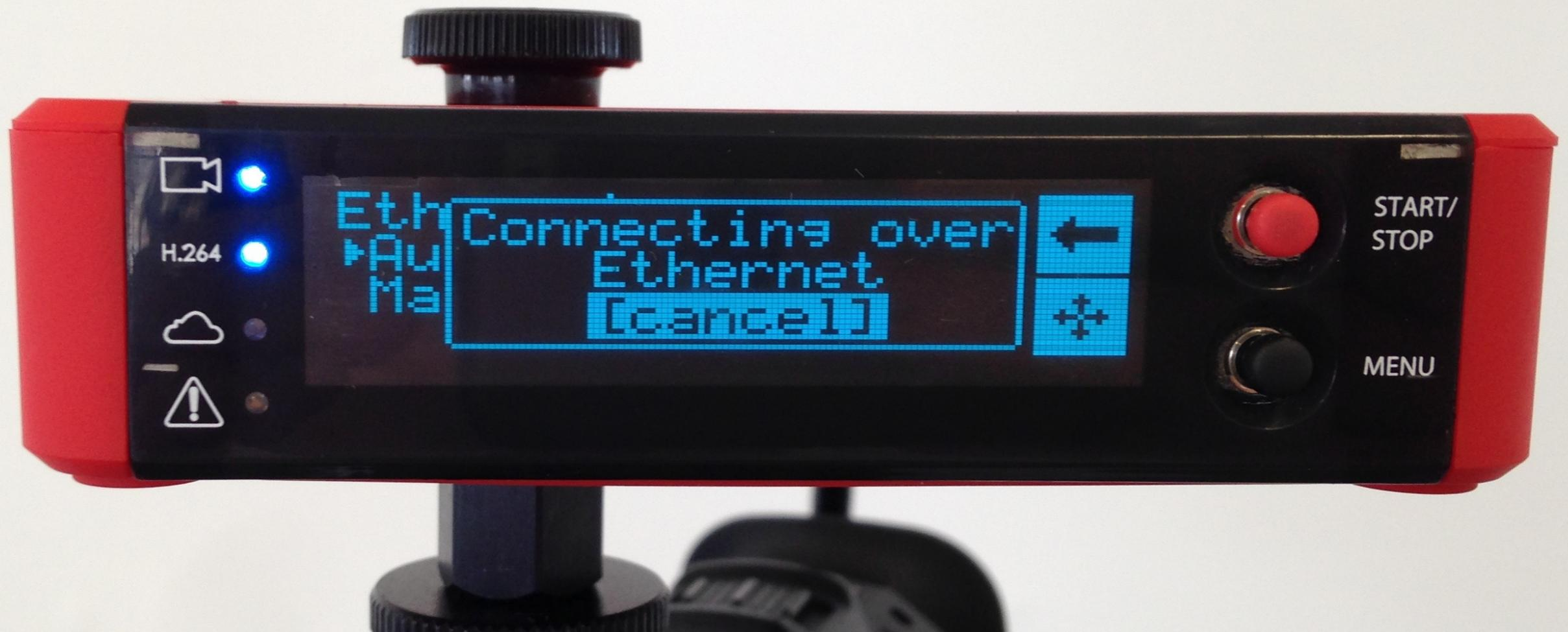
'Automatic (DHCP)' will automatically scan and connect you to your network via Ethernet.
