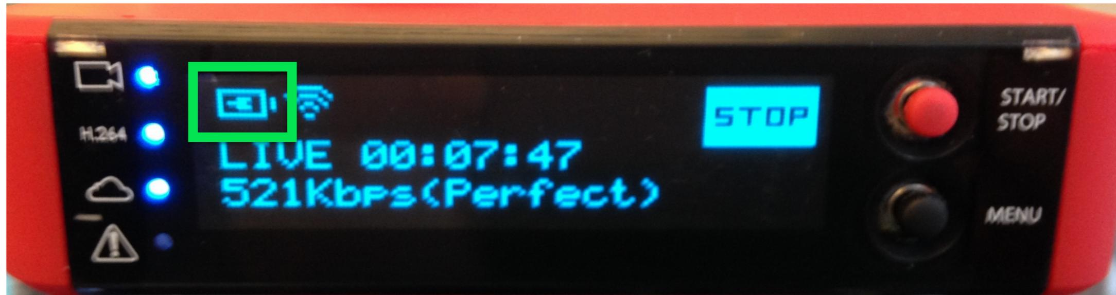
Battery power provides for about three hours of streaming, but you can also stream while the Broadcaster Pro is plugged in.
