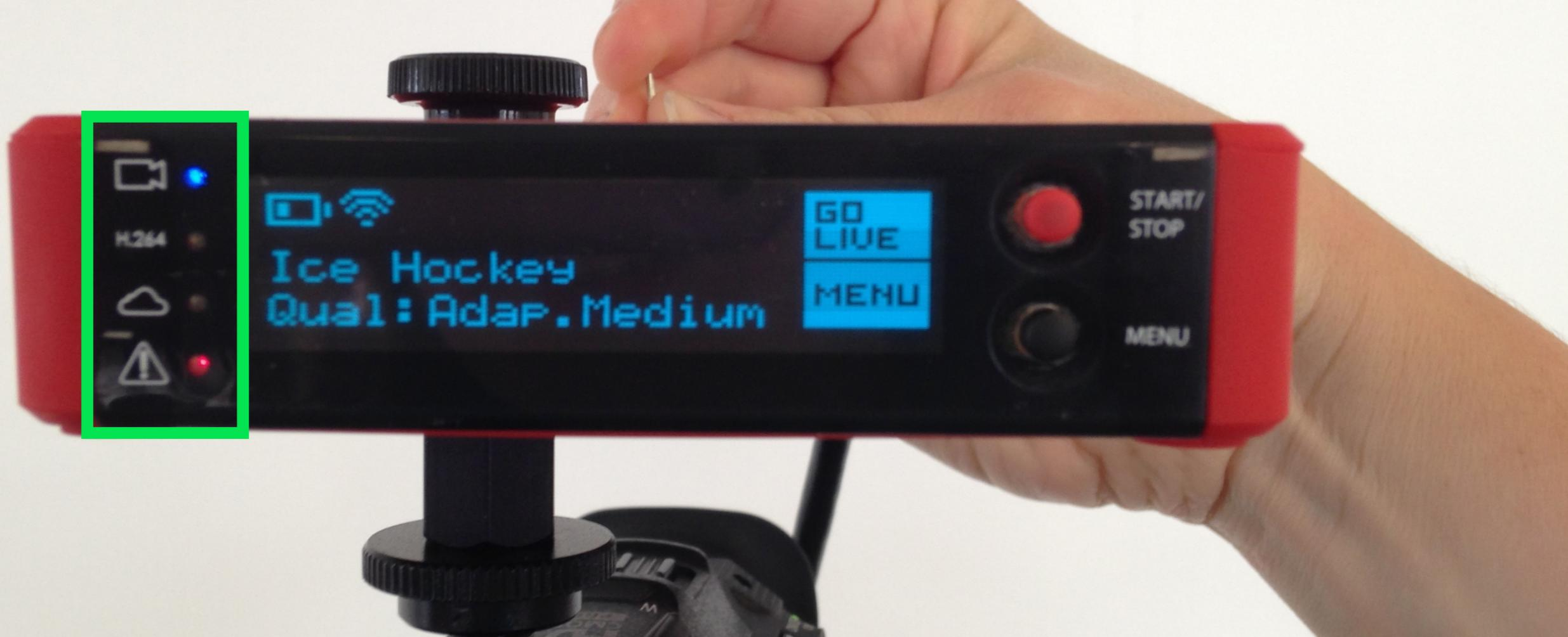
Release the button when you see all four indicator lights switching on and off. The Broadcaster Pro will indicate that it is resetting on the display.
