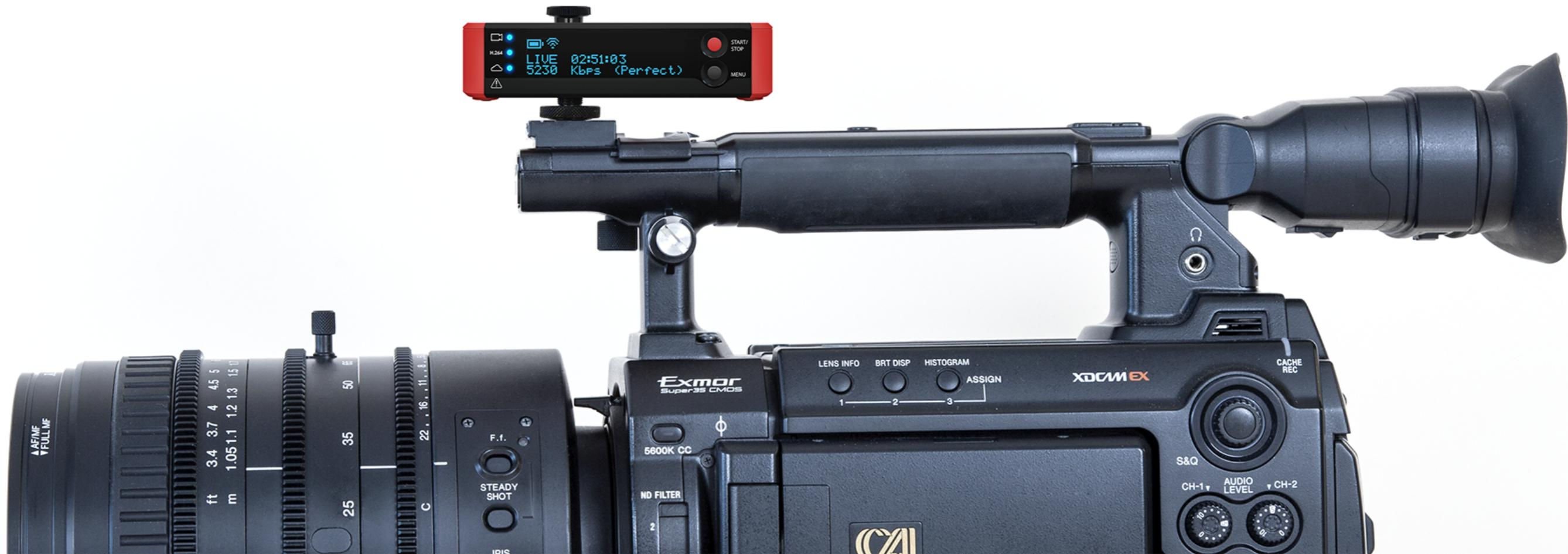
The Broadcaster Pro gives you the ability to stream live directly from any HDMI video source without the need for a PC.
