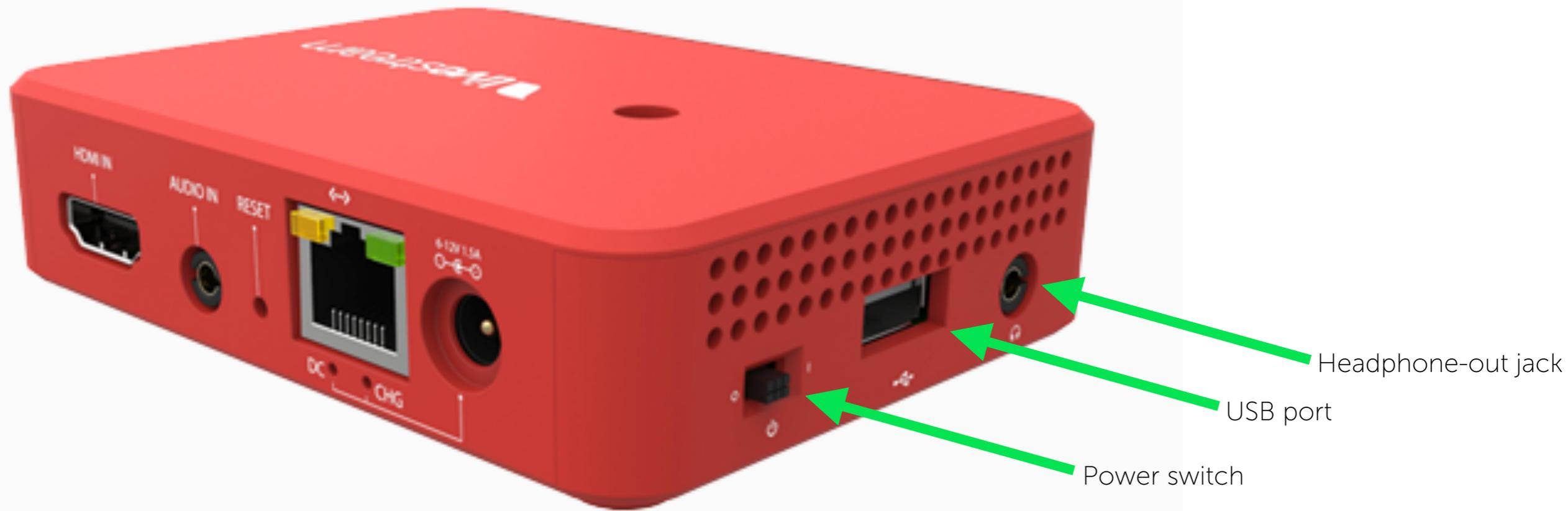
The left side will include the power switch, USB port, and headphone-out jack.
