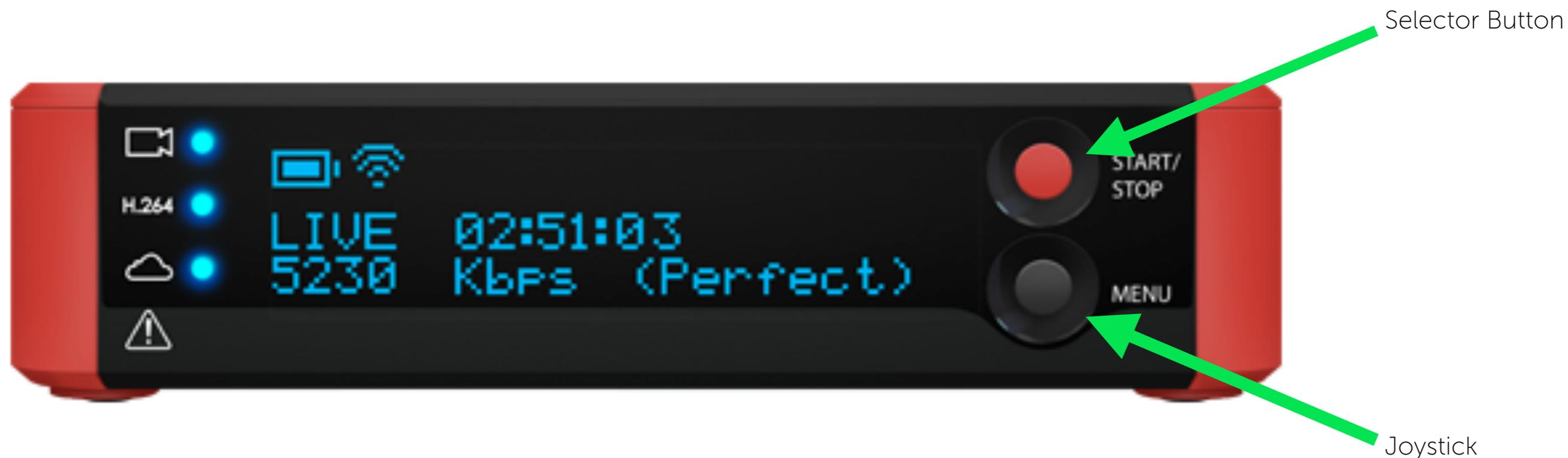
The front of the Broadcaster Pro features an OLED display with a red selector button and black joystick that provide full control of the device.
