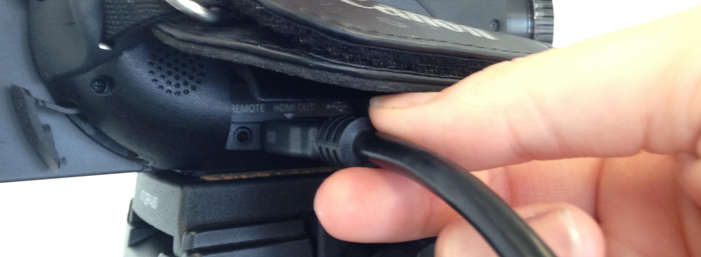
Plug the mini HDMI end of the HDMI cable into your camera.
