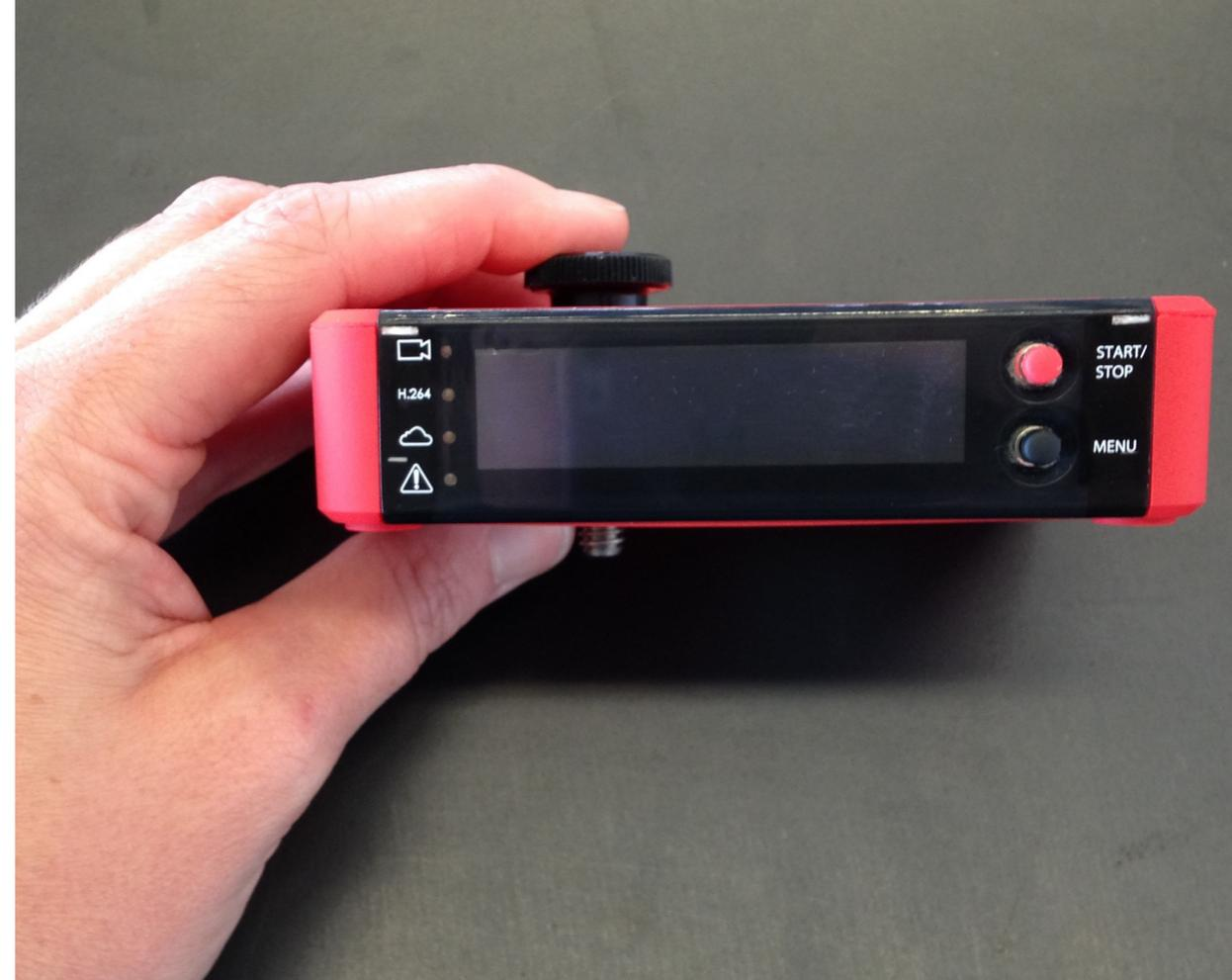
Slide the thumb screw through the hole in the Broadcaster Pro from the top of the device so that the screw side comes out the bottom.
