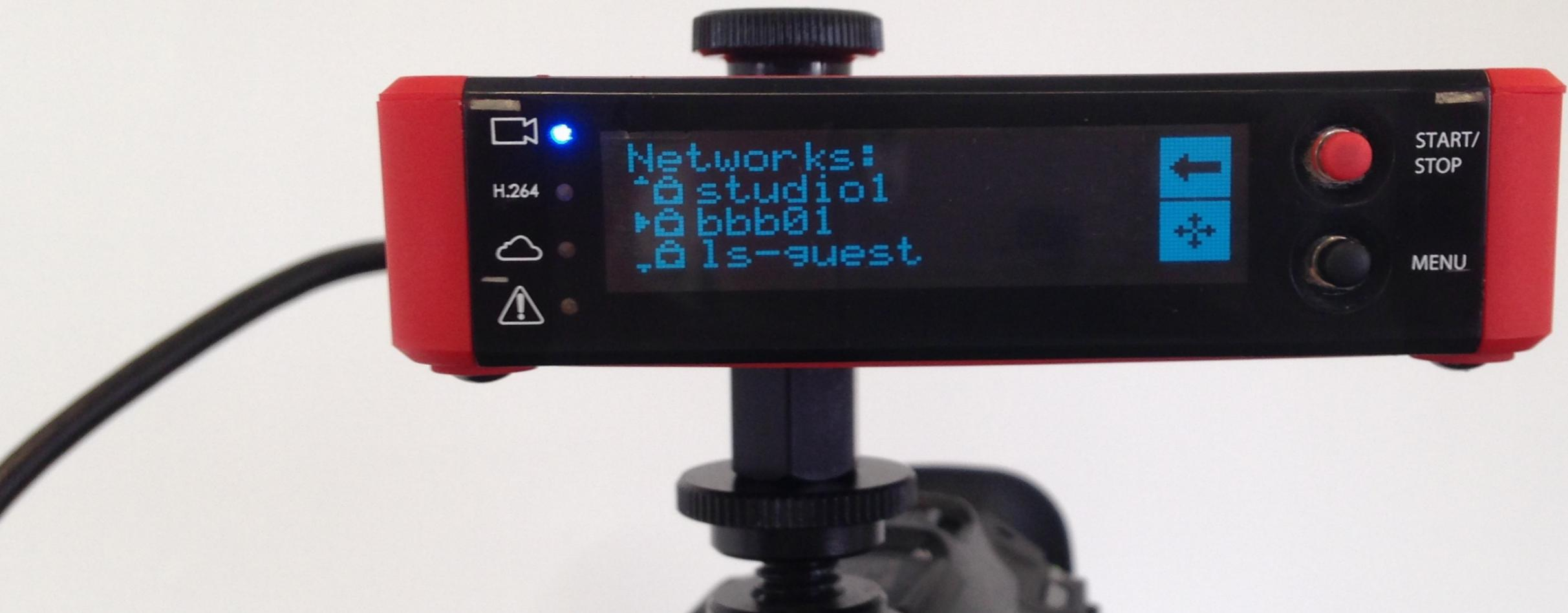
'Scan (SSID)' will scan for Wi-Fi networks within the Broadcastcaster Pro's range and display them. Select your preferred network using the joystick.
