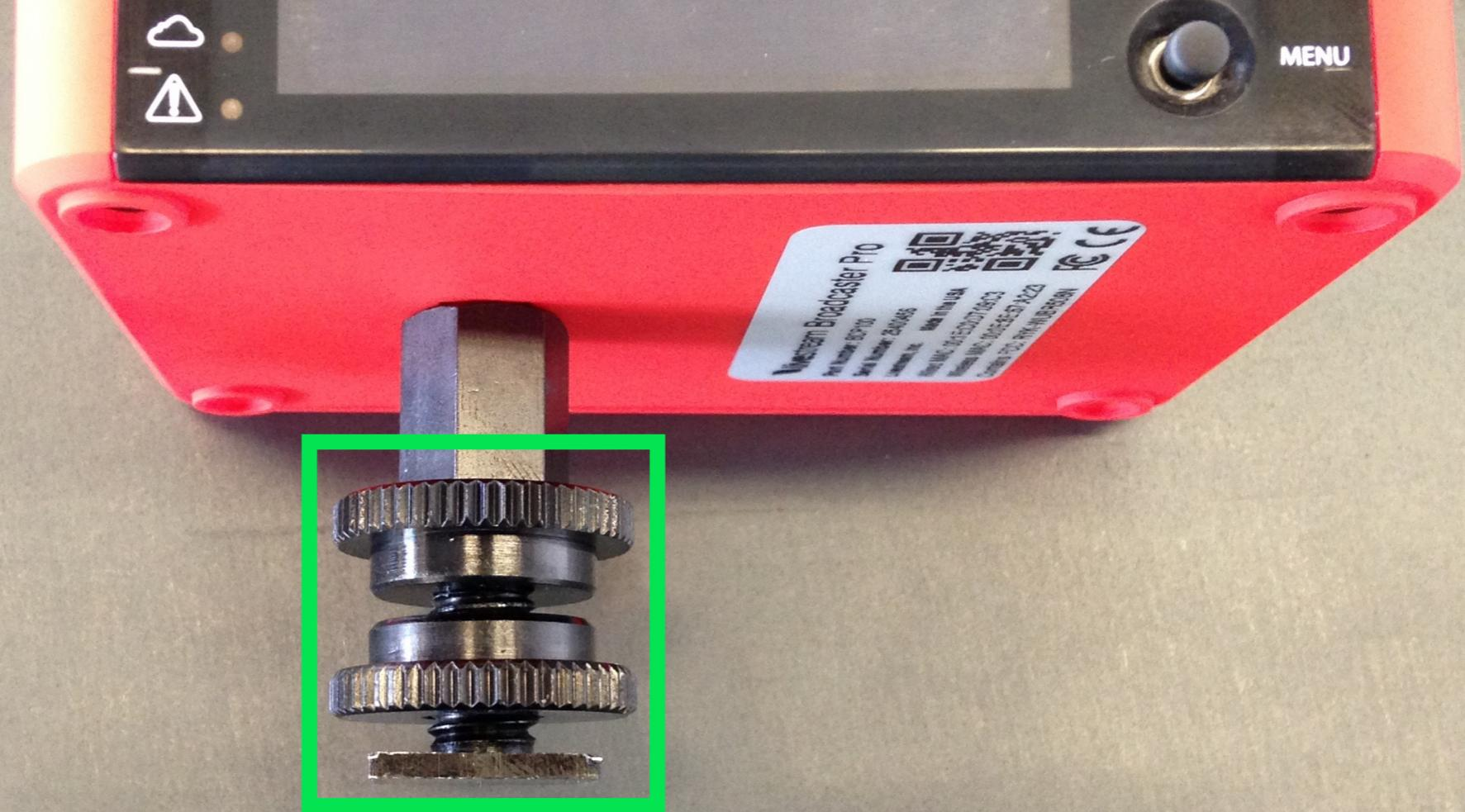
Screw the shoe mount into the nut tightly so that the top washer is touching the bottom of the nut. There should be a small gap between the bottom washer and the mount plate.
