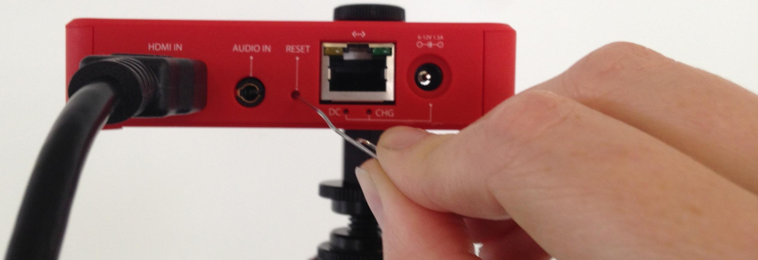
Take a paper clip, pin or similar object and push it into the small reset hole in the back of the Broadcaster Pro while it is powered on for 10-15 seconds.
