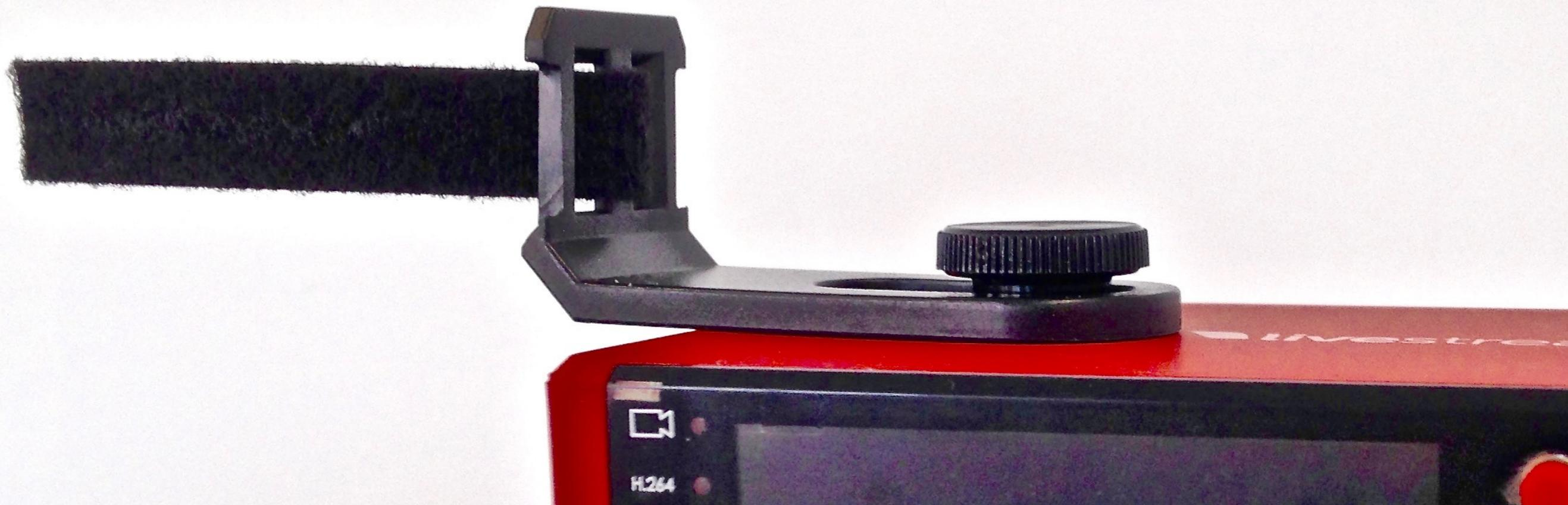
Weave the Velcro strap through the short end of the modem mounting clip, with the strap's soft side facing the Broadcaster Pro.
