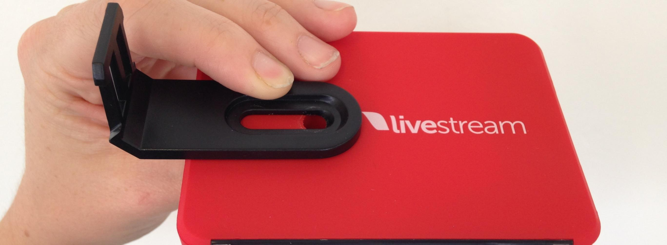
Place the long side of the modem mounting clip on top of the Broadcaster Pro so that the opening lines up with the hole on the device and the short end of the clip is facing upwards.
