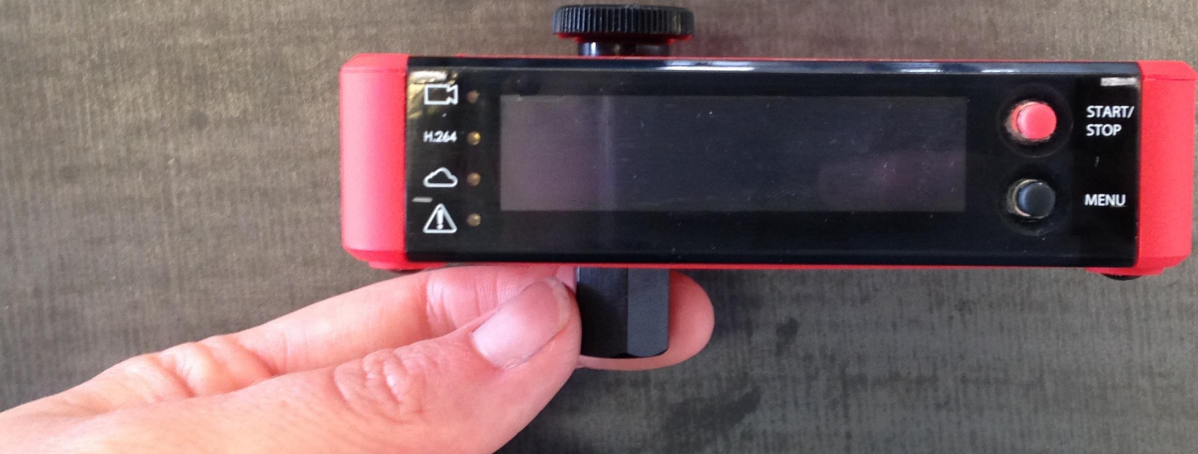
Fasten the nut tightly to the bottom of the Broadcastcaster Pro. The top of the nut should touch the bottom of the device.
