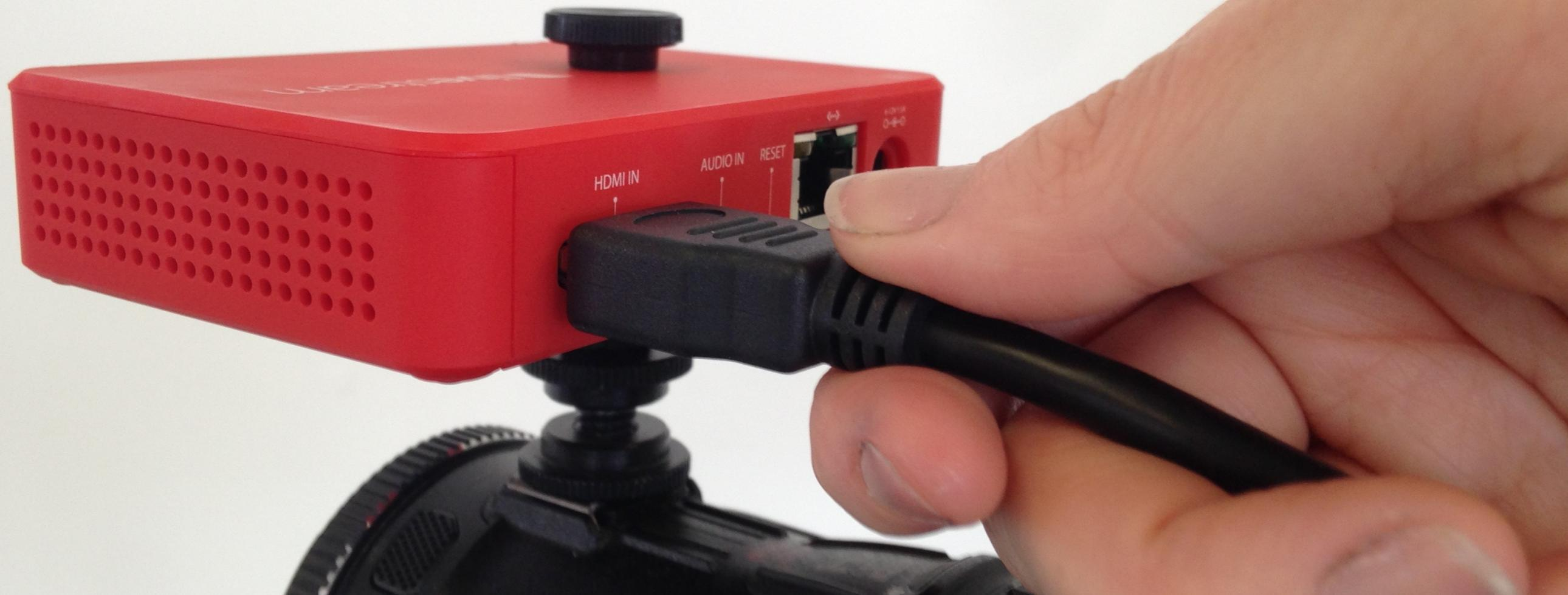
Plug the full-size HDMI end of the HDMI cable into the back of the Broadcaster Pro.
