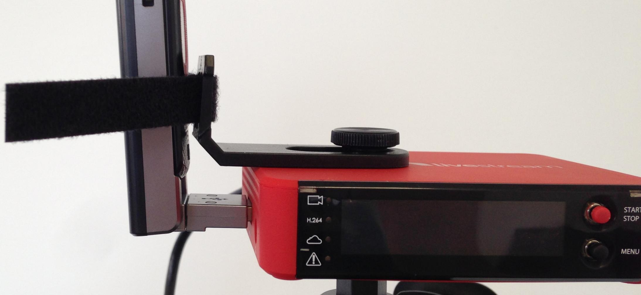
Plug your USB modem into the USB port on the side of the Broadcaster Pro and prop it up against the mounting clip; you may need to adjust the clip, depending on the modem's design.
