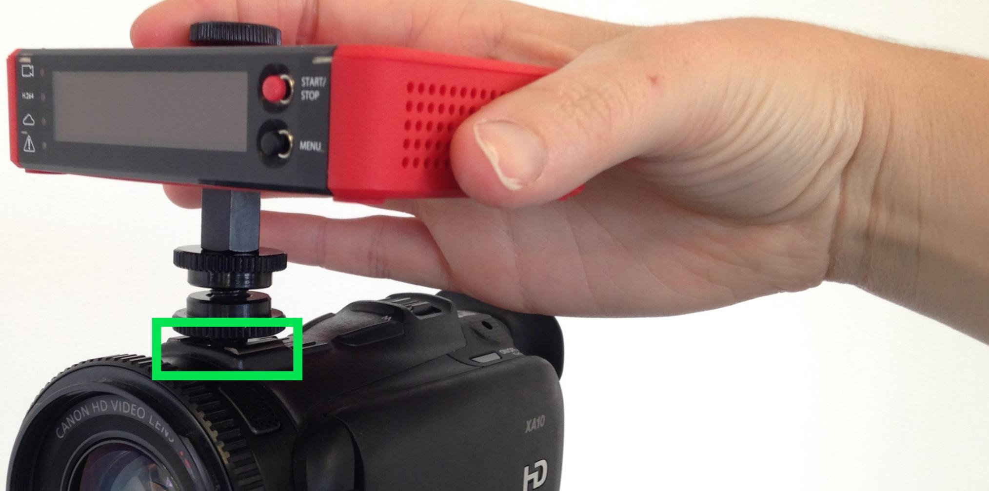
Slide the shoe mount into the shoe on top of your camera, then screw the bottom washer down to secure it against the camera.
