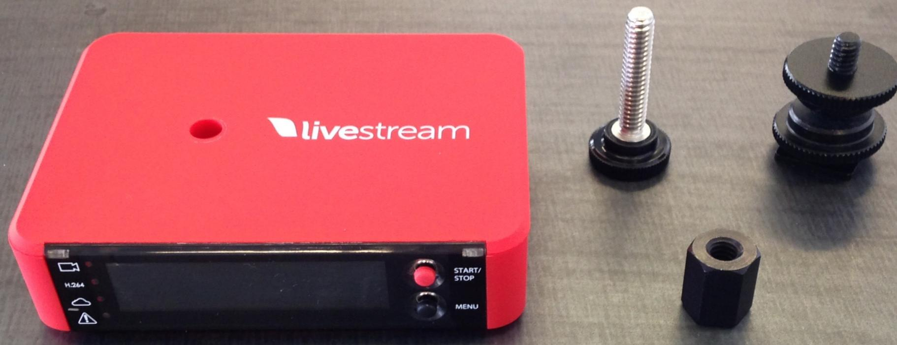
Next, you will need to use the thumb screw, nut, and shoe mount to secure the Broadcaster Pro on top of your camera.
