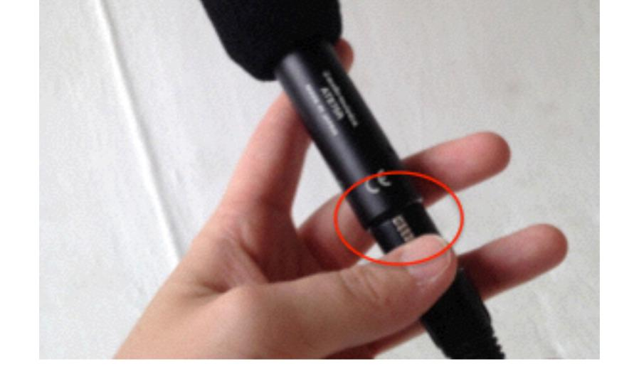
Push the cable and microphone together, holding down the silver metal clasp to secure the connection.
