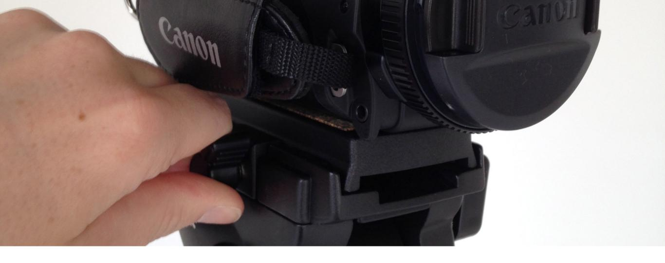
Once the plate is settled on the tripod, turn the black knob on the side of the tripod to secure the camera's placement.
