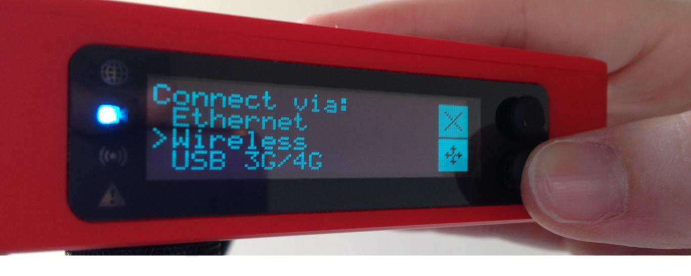
You will need to connect Livestream Broadcaster to the Internet. Ethernet is recommended when possible. Use the bottom joystick to toggle to either Wireless or 3G/4G when necessary.
