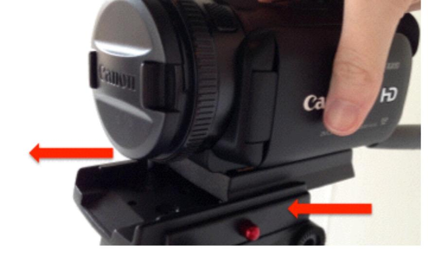
Now slide the camera on top of the tripod. You'll likely need to hold down the release button in order to get the entire plate on top of the tripod.
