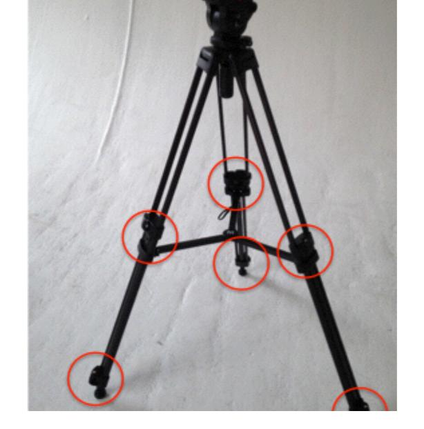
The first part of setting up any camera shoot is usually the tripod. Raise your tripod to the desired height by unlocking and expanding the legs.
