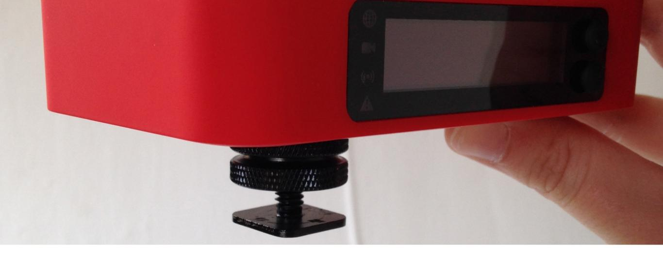
Screw in the shoe mount to the bottom of Livestream Broadcaster until it is secure.
