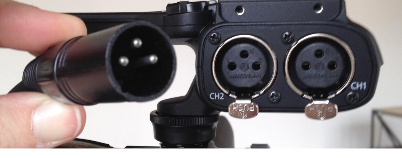
Now take the male end of the XLR cable and match it up to one of the corresponding XLR inputs (on this camera, they can be found on the handle unit).
