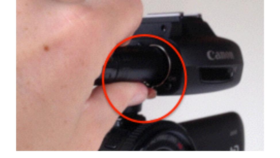
Hold down the metal clasp on the input and plug in the XLR cable.
