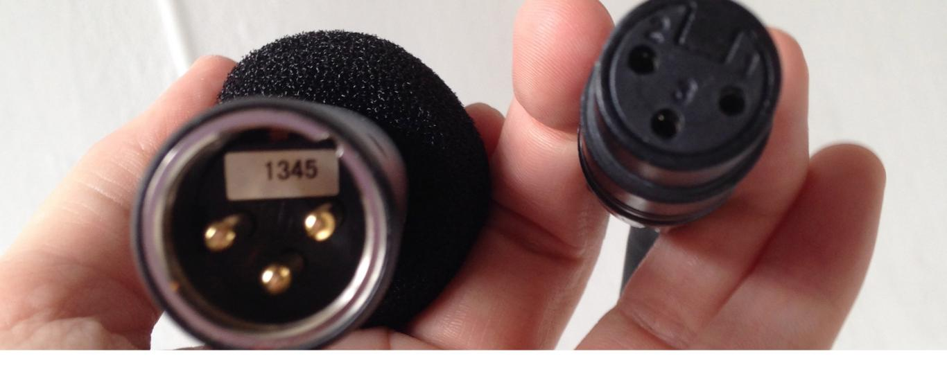
Notice that the bottom of your microphone has prongs that match the female end of the XLR cable.
