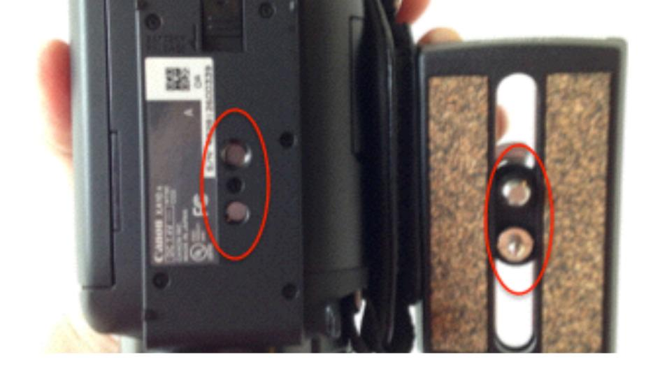
Notice that the two screws on the bottom of the plate match the size of the screw holes on the bottom of your camera. This is how you will attach them.
