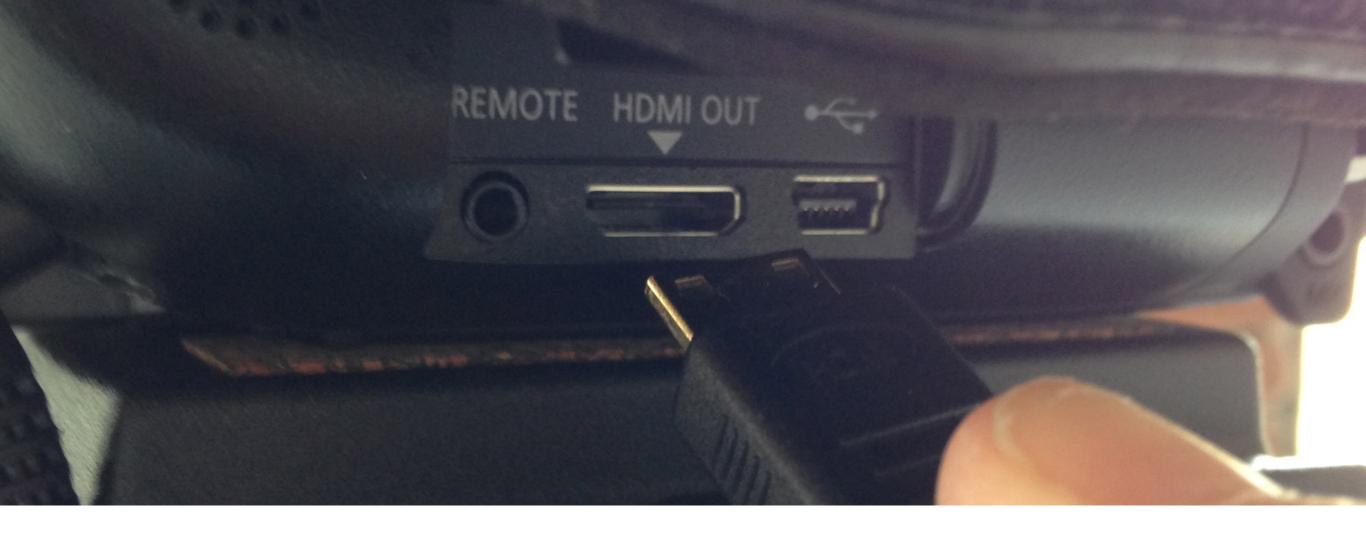
Take the HDMI cable that came with Livestream Broadcaster and plug it into your camera's HDMI output port.
