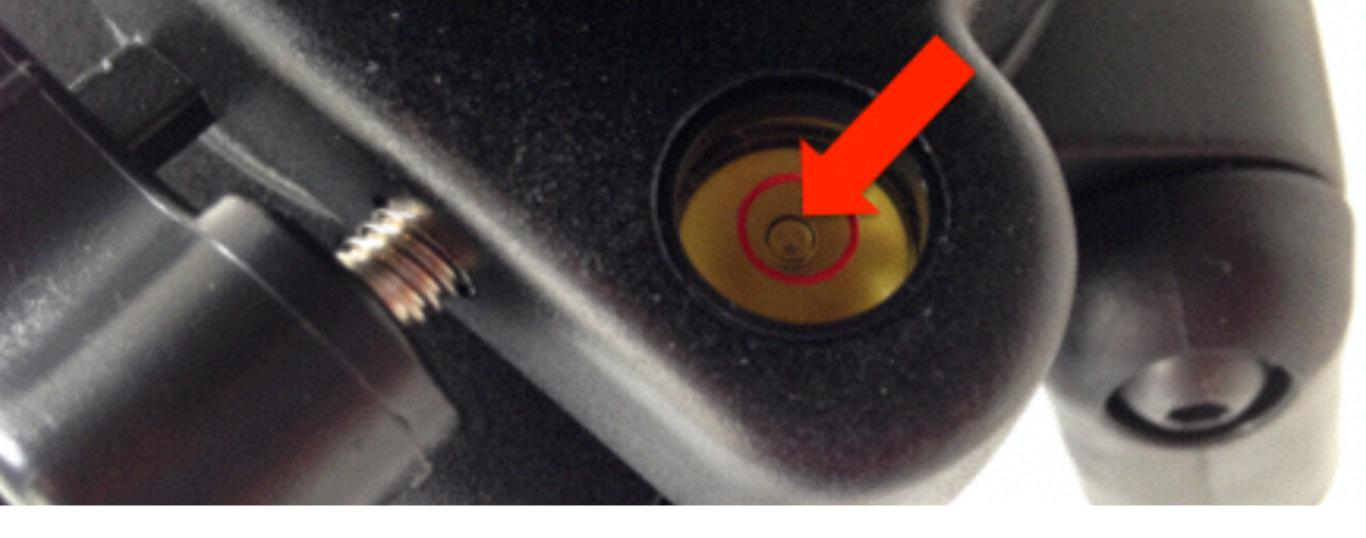
To make sure your tripod is level, check the bubble indicator toward the top. Make sure the bubble is completely inside the circle, then lock the legs of the tripod.
