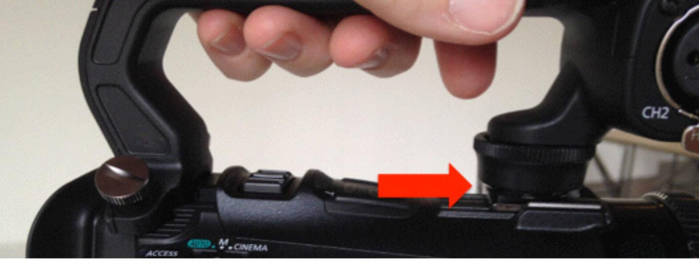
Slide the handle into the mount on top of the camera.
