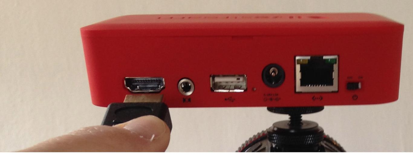
Now connect the other end of the HDMI cable to the HDMI input port on the back of Livestream Broadcaster.
